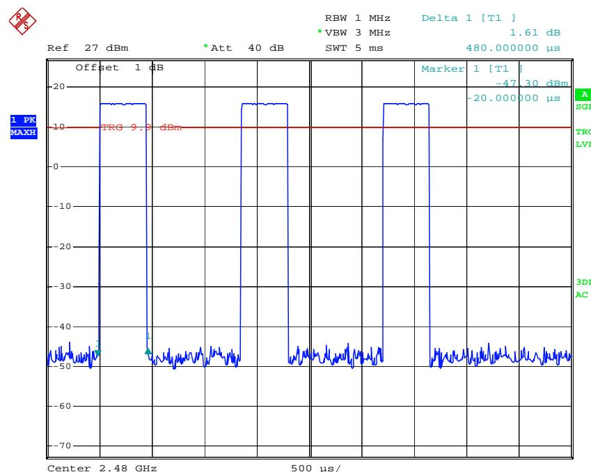
**FCC §15.247(b) (1) - PEAK OUTPUT POWER MEASUREMENT****Applicable Standard**
