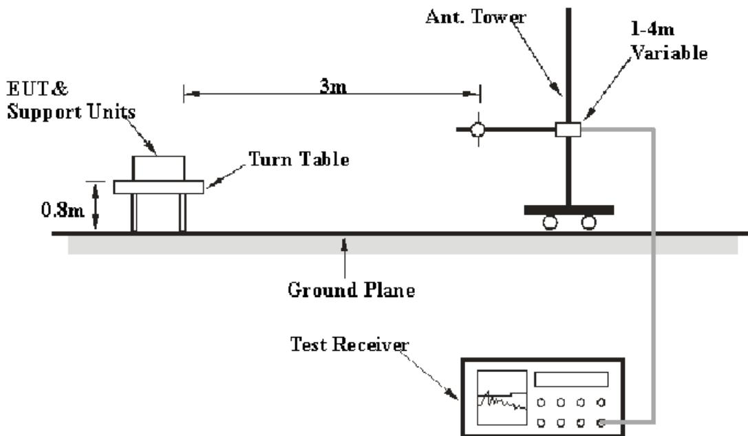
The radiated emission tests were performed in the 3 meters, using the setup accordance with the ANSI C63.4-2009. The specification used was the FCC 15.209, and FCC 15.247 limits.
