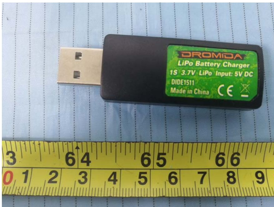
EUT – Battery Charger View
