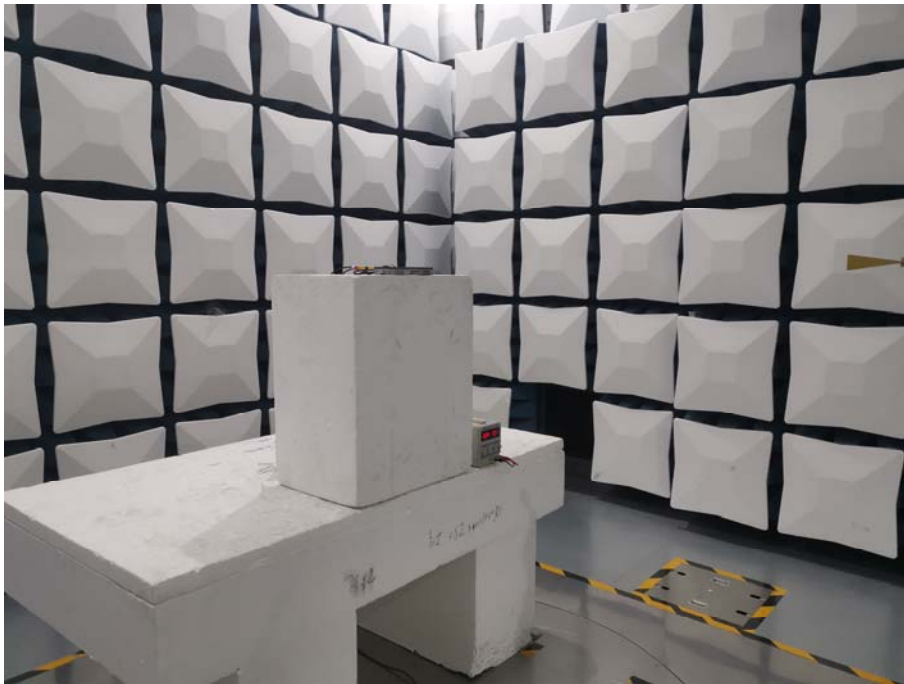
Radiated Spurious Emissions Test View (50-75GHz)
