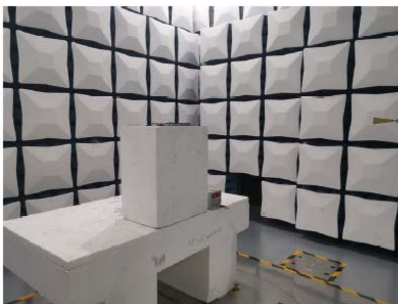
Radiated Spurious Emissions Test View (50-75GHz)
