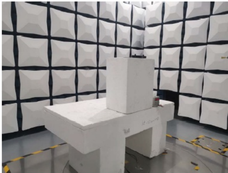
Radiated Spurious Emissions Test View (90-100GHz)
