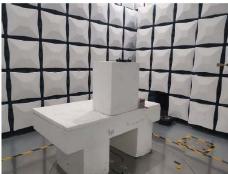
Radiated Spurious Emissions Test View (50-75GHz)
