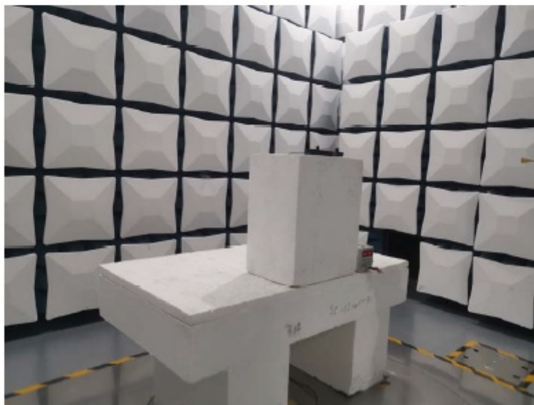
Radiated Spurious Emissions Test View (90-100GHz)
