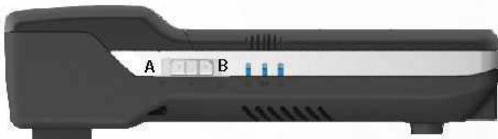
Figure 1-1: Network-Attached Storage Switch Indication
