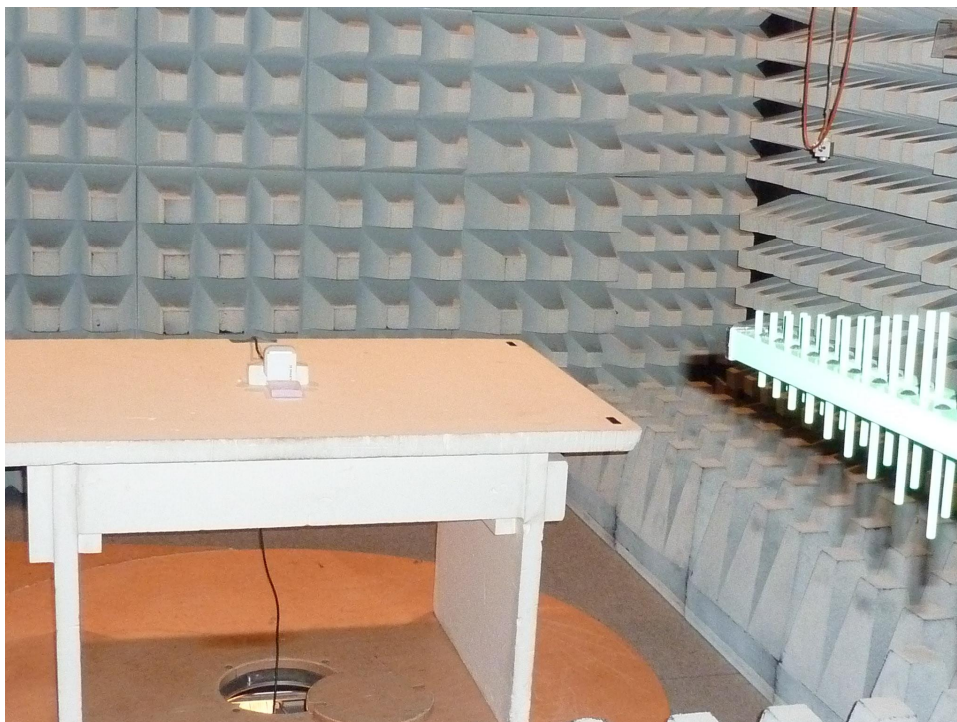
181073emi3.JPG: Radiated emissions FAR > 30MHz
