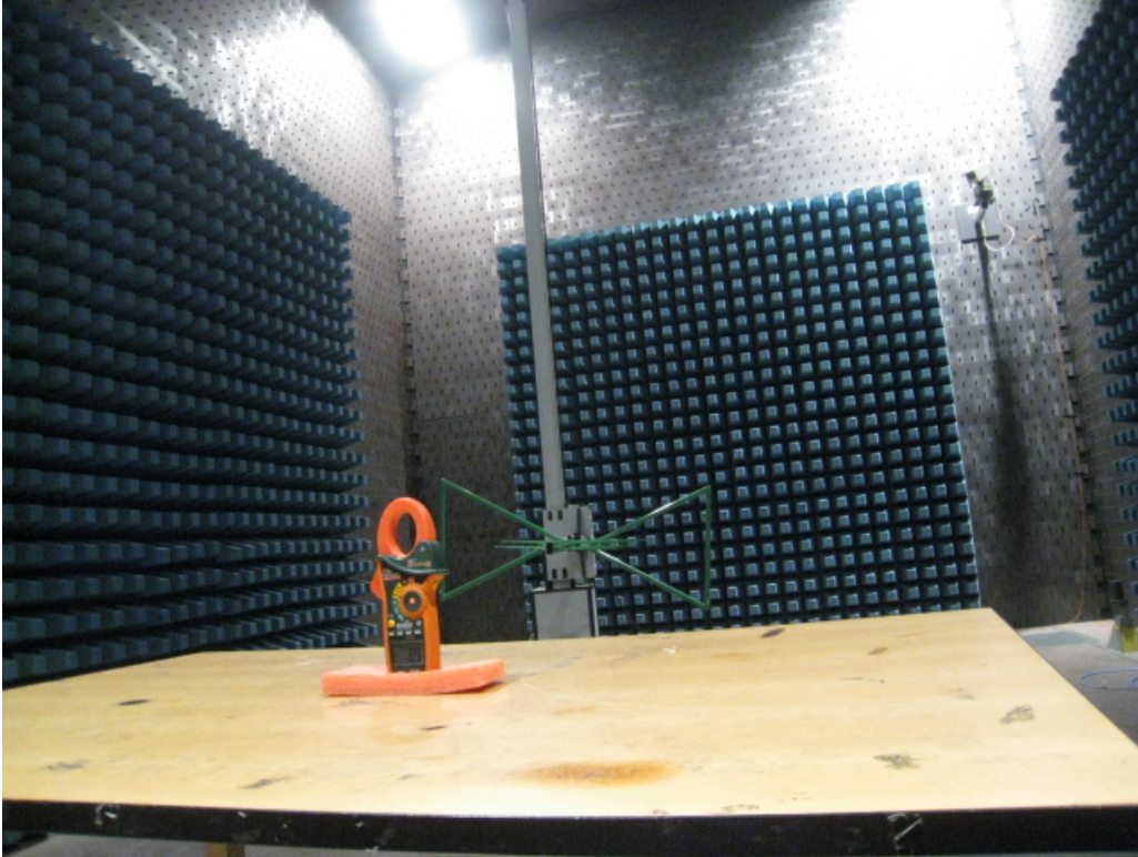
Photo 1 Front of Radiated Disturbance Test (Below 1GHz)
