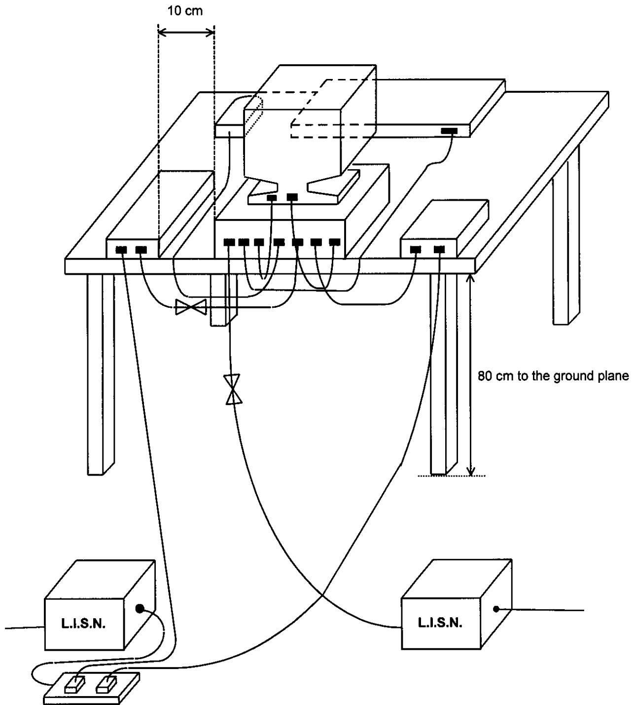
**5.4. TEST RESULT OF AC POWERLINE CONDUCTED EMISSION**
