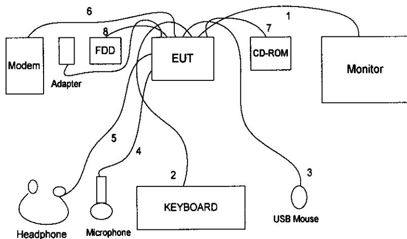
1. The I/O cable is connected from EUT to the support device 1.
