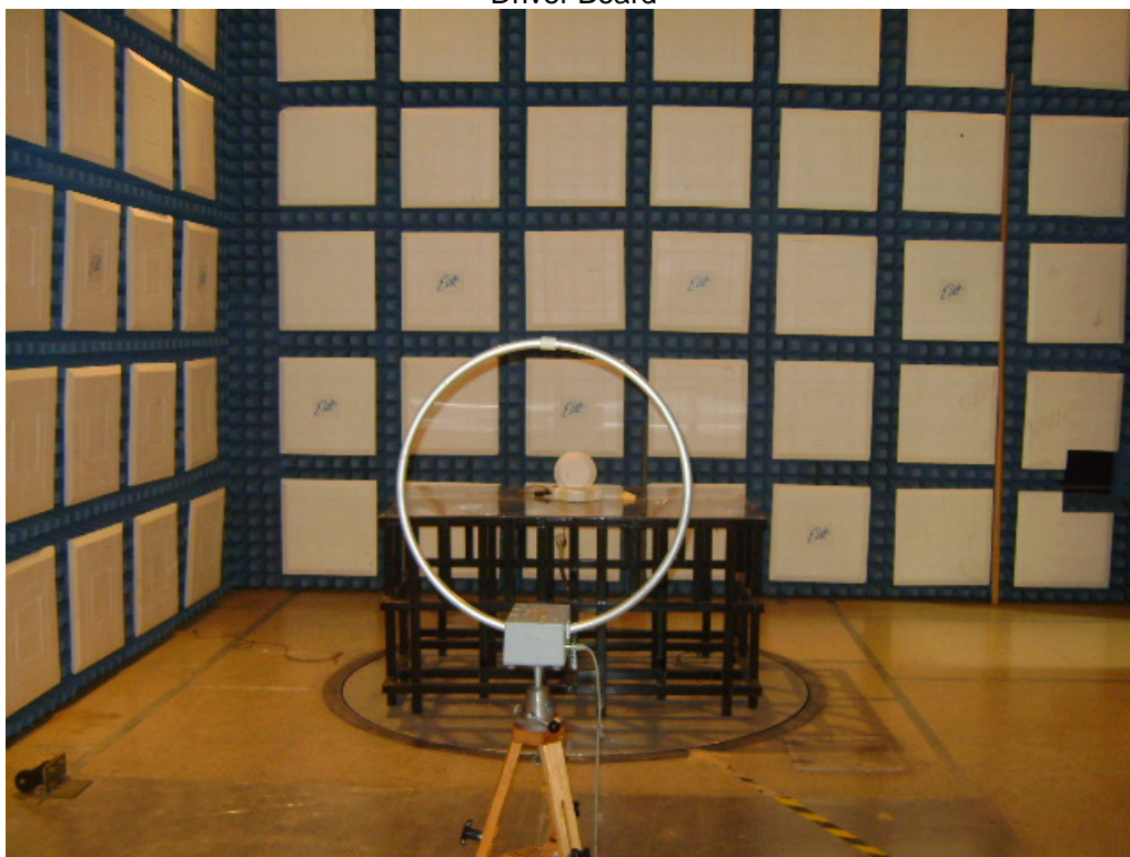
Test Setup for Radiated Emissions – Vertical Polarization, Integrated Antenna Driver Board
