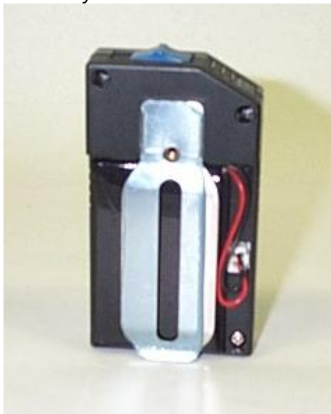
Battery – Rear Cover Removed
