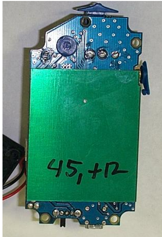
Main Board – Foil side with ground plane removed
