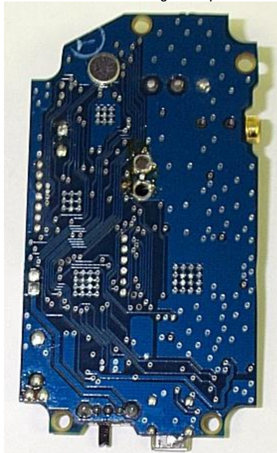
Main Board – Foil side with ground plane removed
