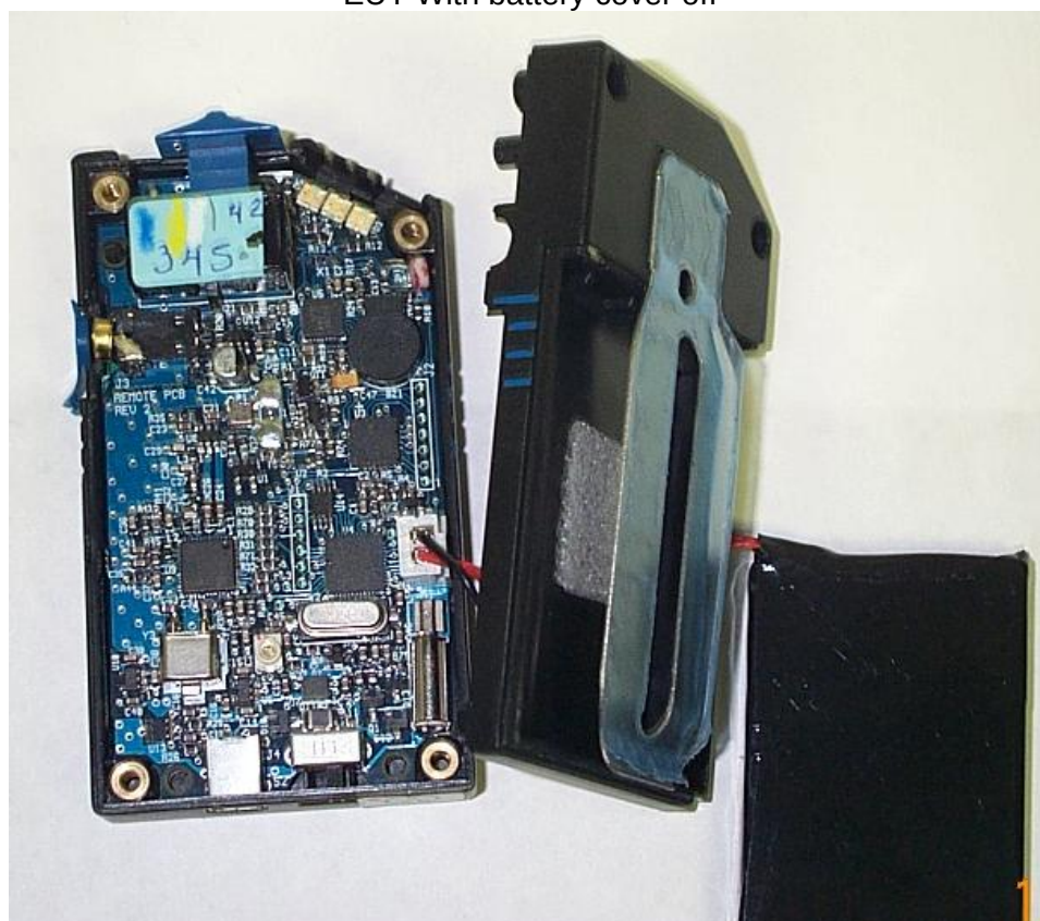
EUT With battery cover off
