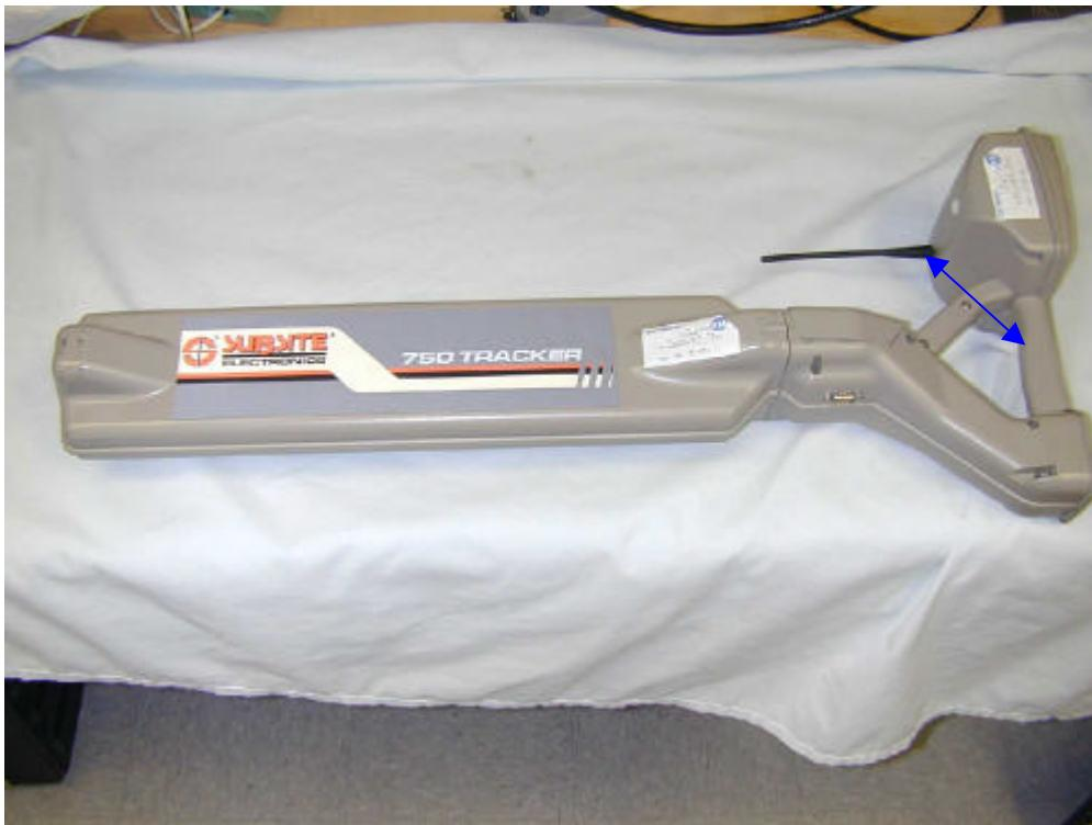
>10 cm. From closest part of handle to closest part of antenna. The orientation of the LCD display dictates that the user operate the EUT with the antenna away from the body in order to be able to read the display.
