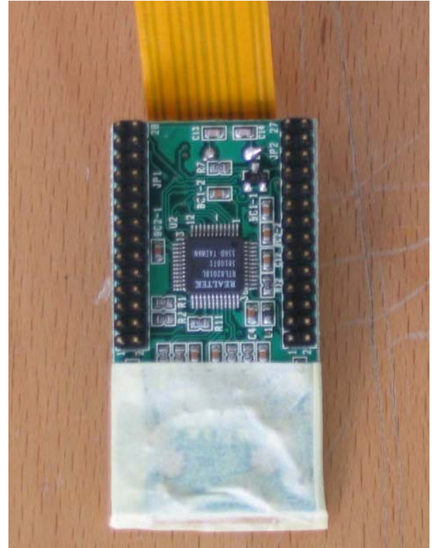
Fig. 3: LAN interface board - top side (left) and bottom side (right)
