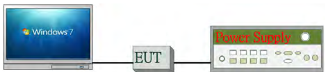
Fig. 2-1 Radiated & Conducted (Antenna Port) Emission Configuration
