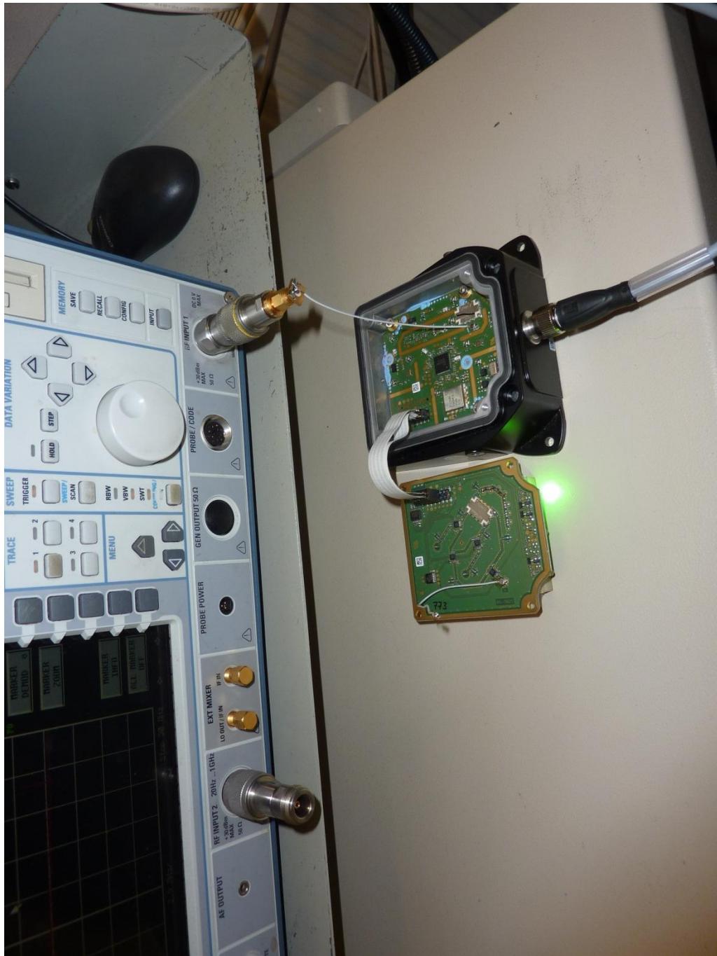
136258_f.JPG: IUH-F190-V1-FR2-02, test set-up conducted rf-tests
