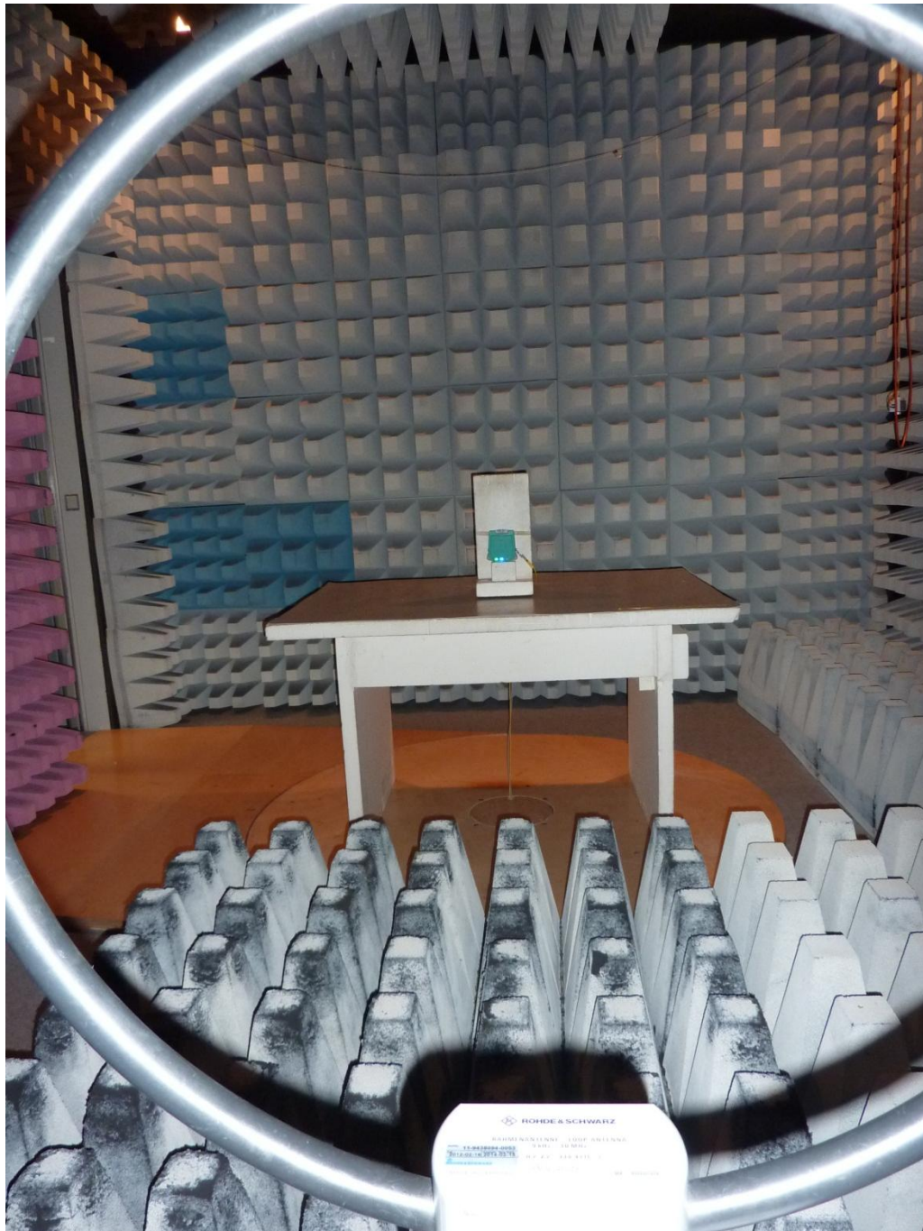
136258_e.JPG: IUH-F190-V1-FR2-02, test set-up fully anechoic chamber
