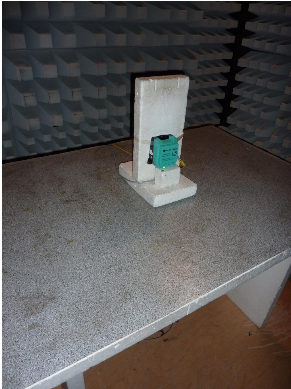
136258_b.JPG: IUH-F190-V1-FR2-02, test set-up fully anechoic chamber
