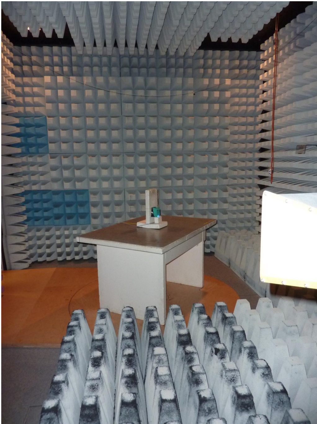
136258_d.JPG: IUH-F190-V1-FR2-02, test set-up fully anechoic chamber
