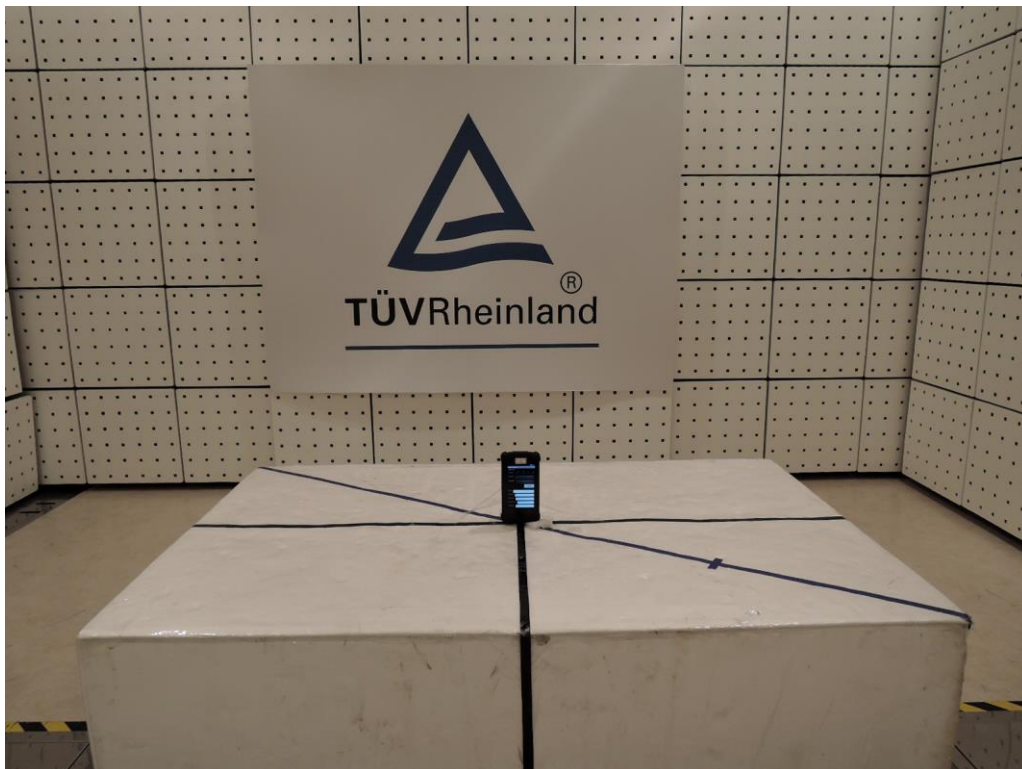
Photograph 1: Set-up for Spurious Emissions (Front View)
