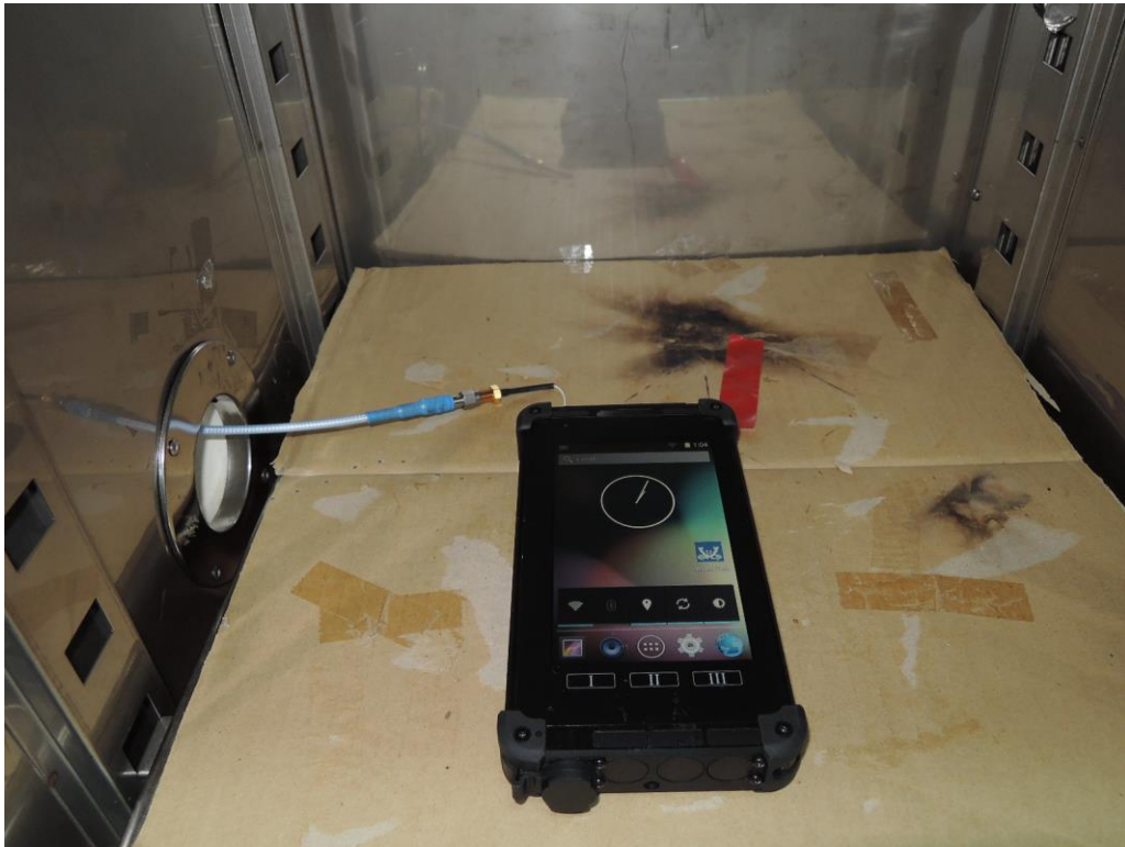
Photograph 4: Set-up for Conducted testing
