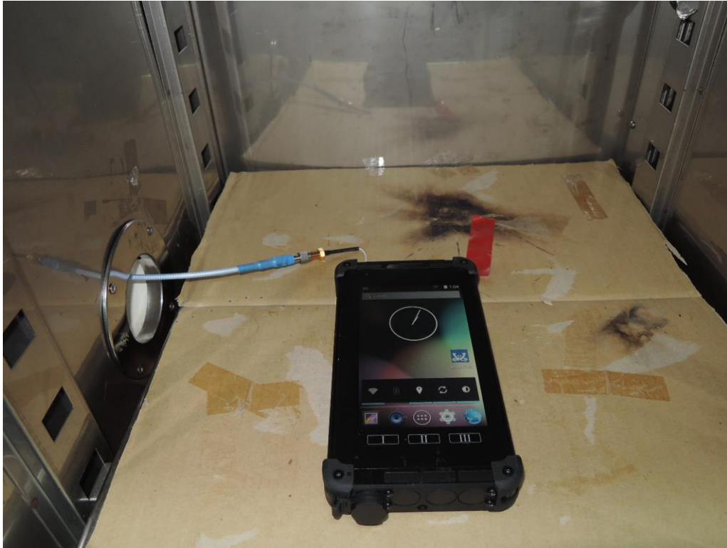
Photograph 5: Set-up for for Mains Conducted testing Back
