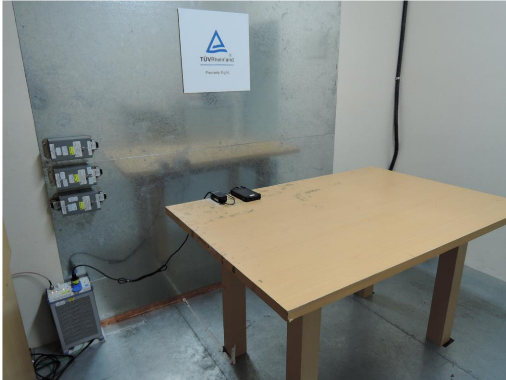
Photograph 6: Set-up for for Mains Conducted testing Front
