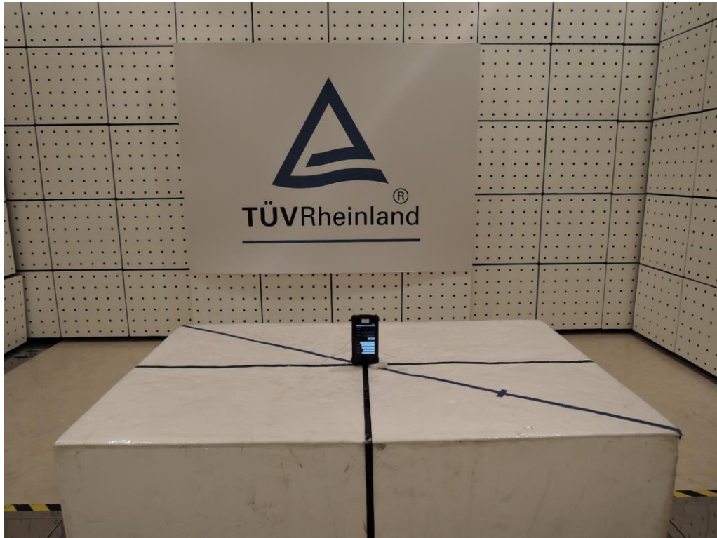
Photograph 1: Set-up for Spurious Emissions (Front View)
