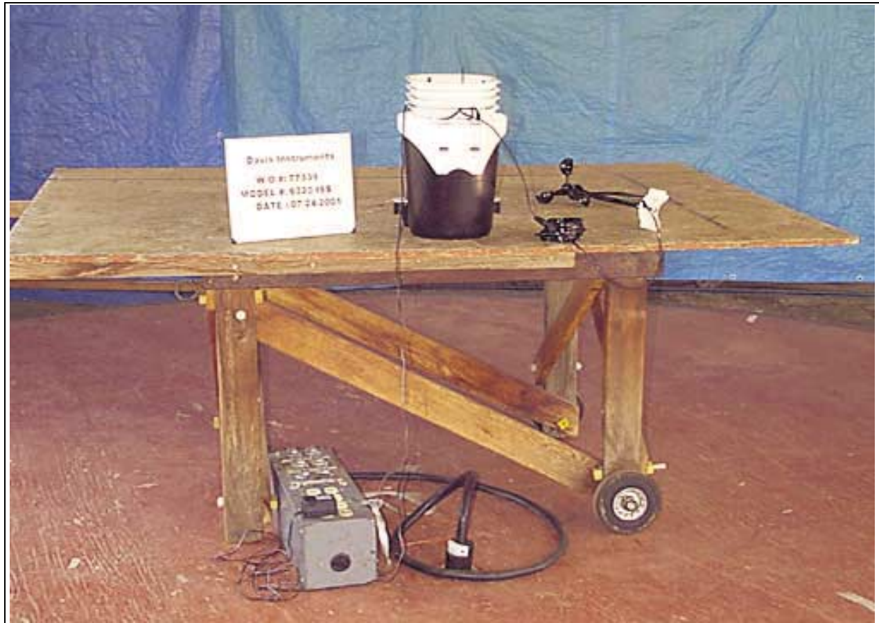
Radiated Emissions - Back View of Integrated Sensor Suite, 6320
