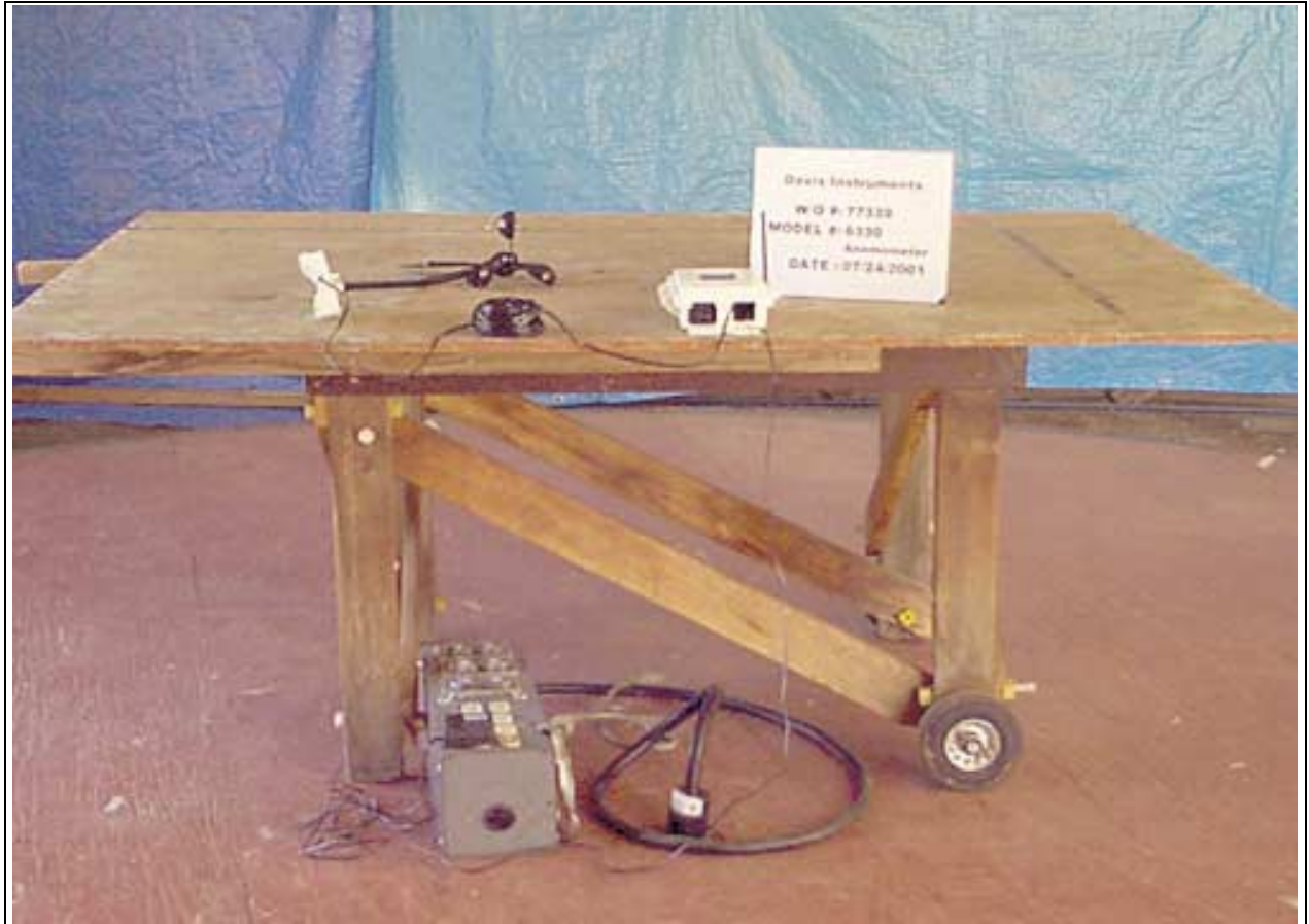
Radiated Emissions - Back View of Anemometer Transmitter Kit, 6330
