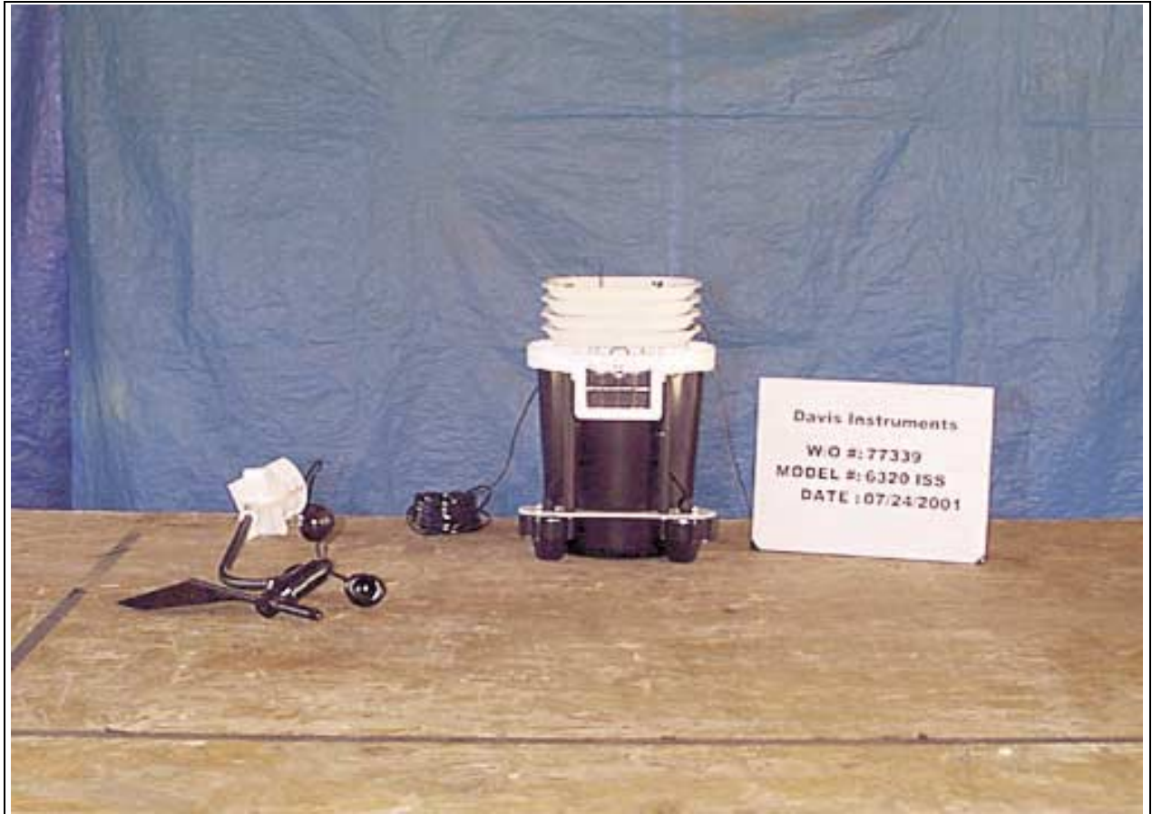
Radiated Emissions - Front View of Integrated Sensor Suite, 6320
