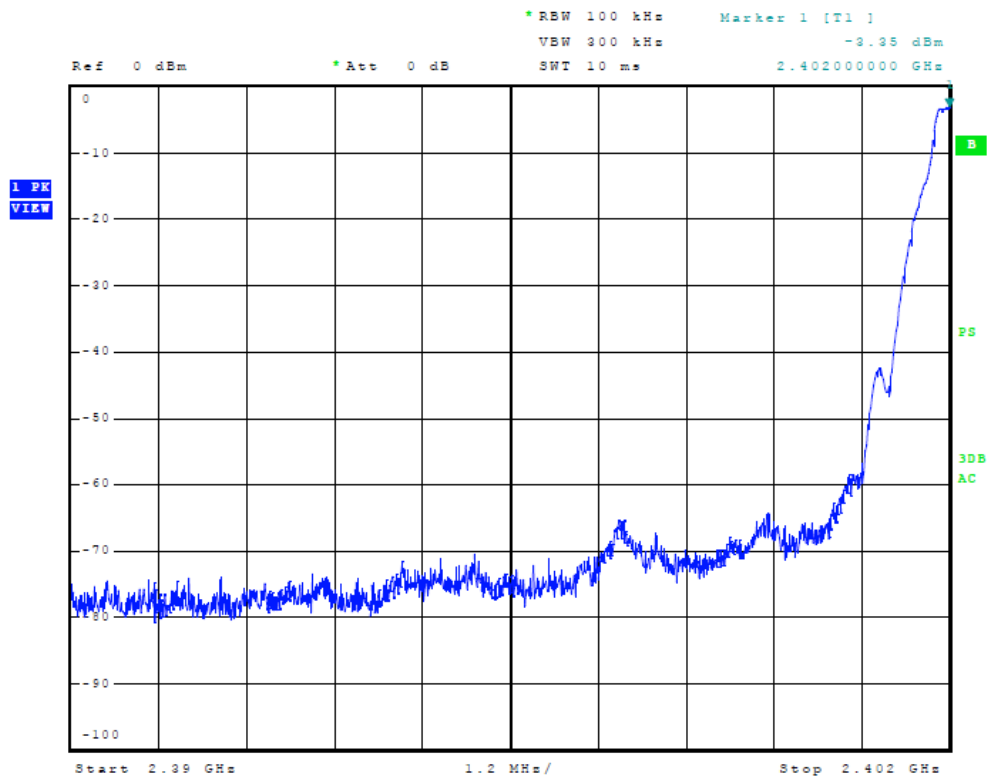
Figure 7 Plot of Transmitter Emissions (Low Band Edge)
