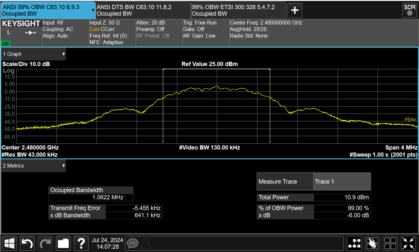
Figure TR10.2: Occupied bandwidth data for BLE 1 Mbps at high channel (2480 MHz)
