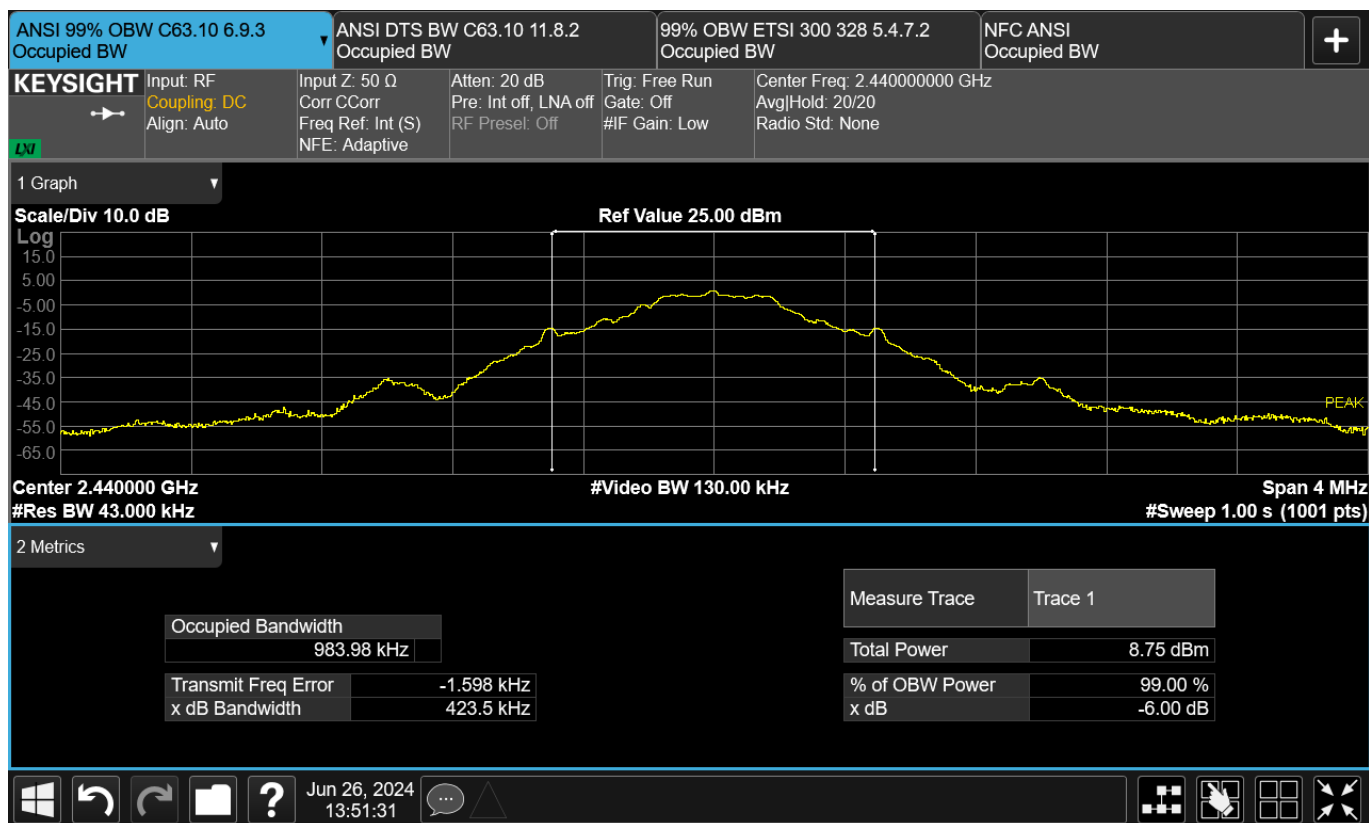
Figure TR10.4: Bandwidth data for ANT at 2440 MHz
