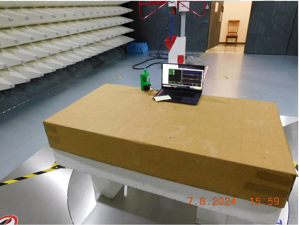
Figure RE09.3: EUT test setup, second view
