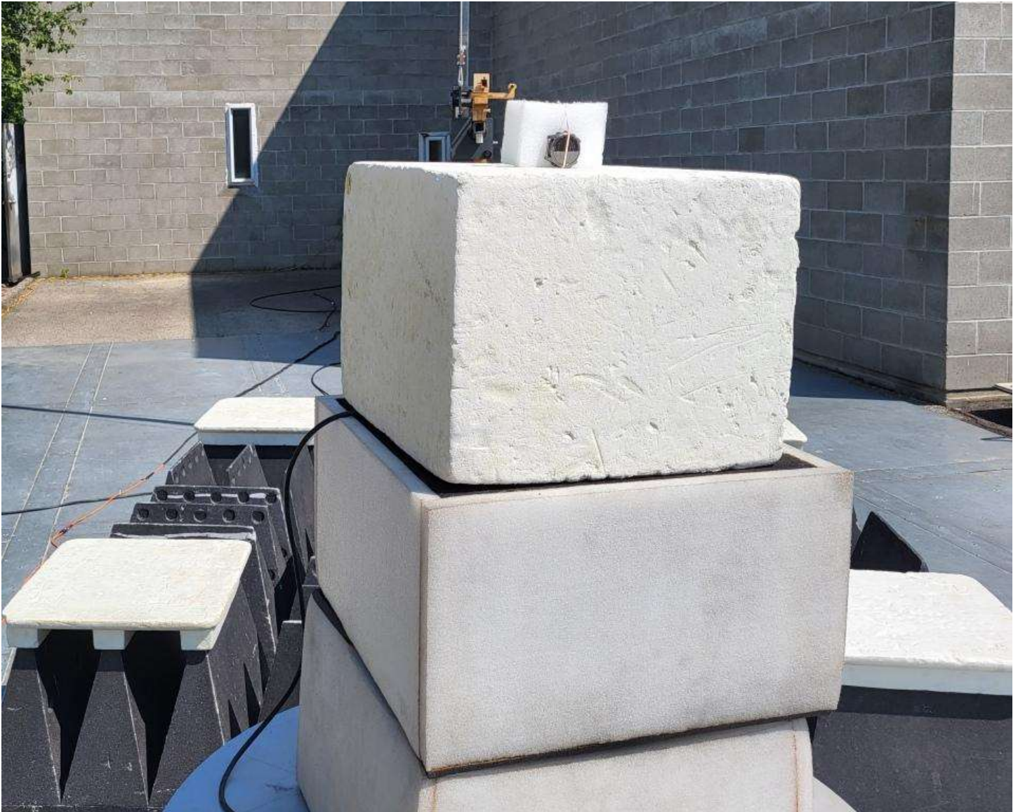
Figure E15.6 – Setup, Radiated Tx Measurements, 18 – 26GHz
