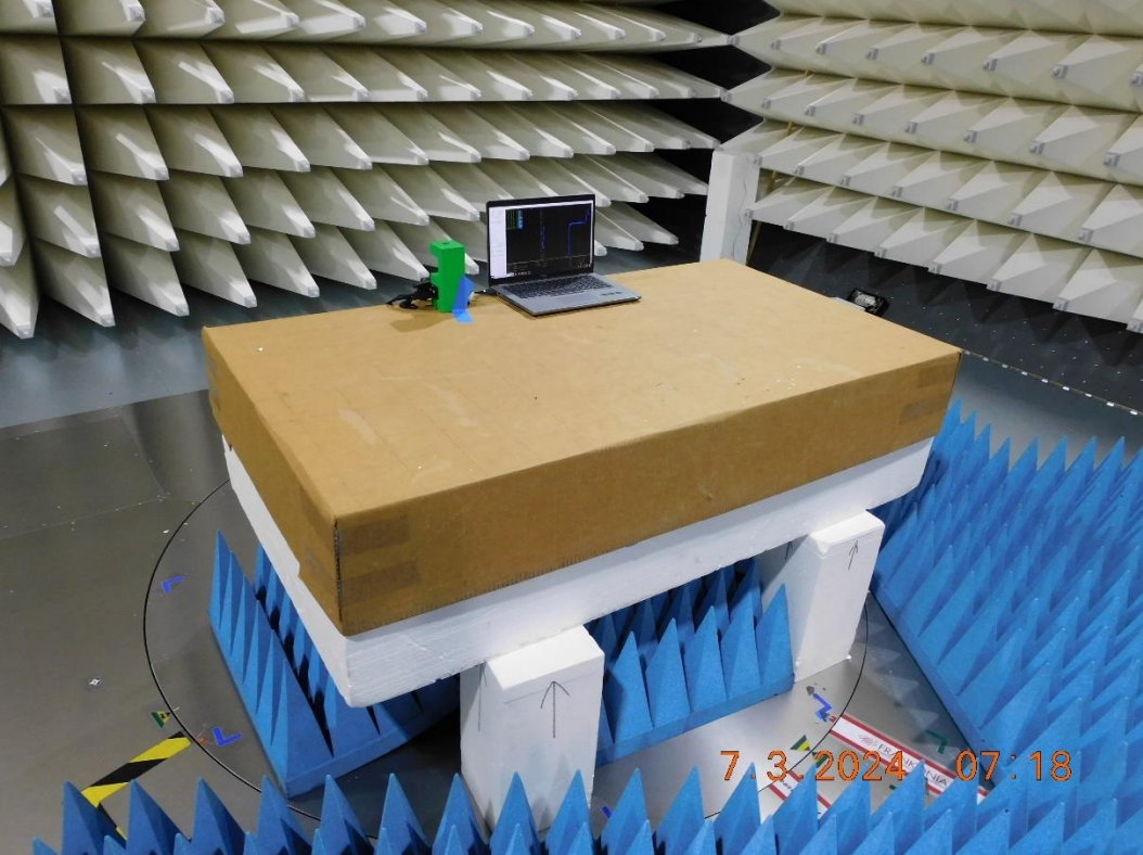
Figure RE11.2: EUT test setup, first view (X orientation)
