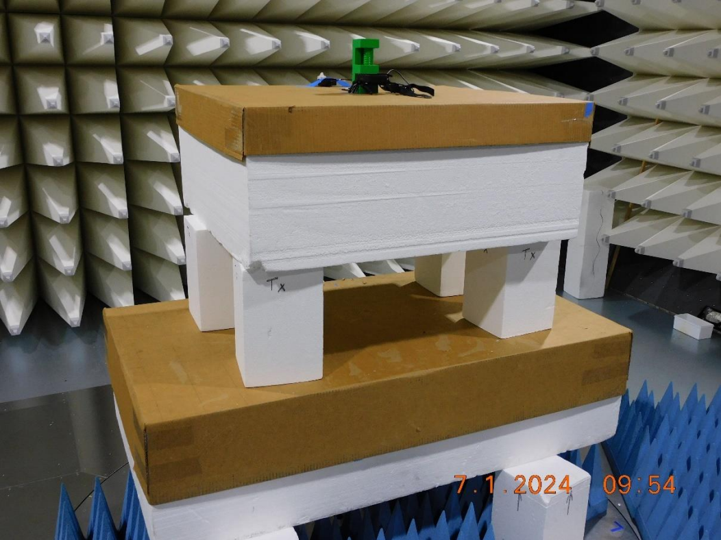
Figure RE01.21: EUT test setup, primary view
