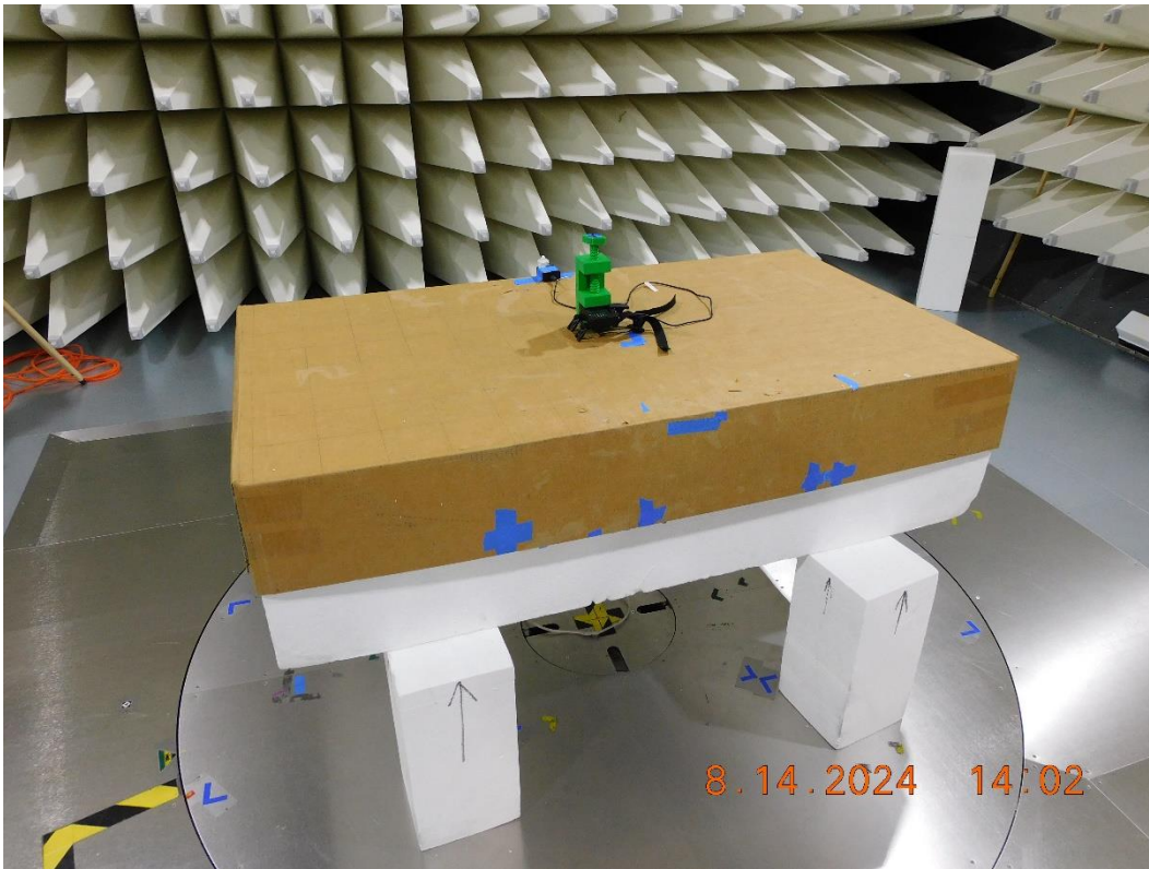
Figure RE30.6: EUT test setup, first view (Antenna Z POL)
