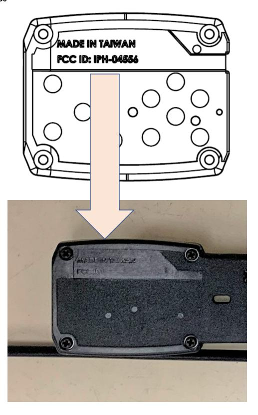
FCC ID will be permanently molded into the flex-band of the dog device as shown above.
