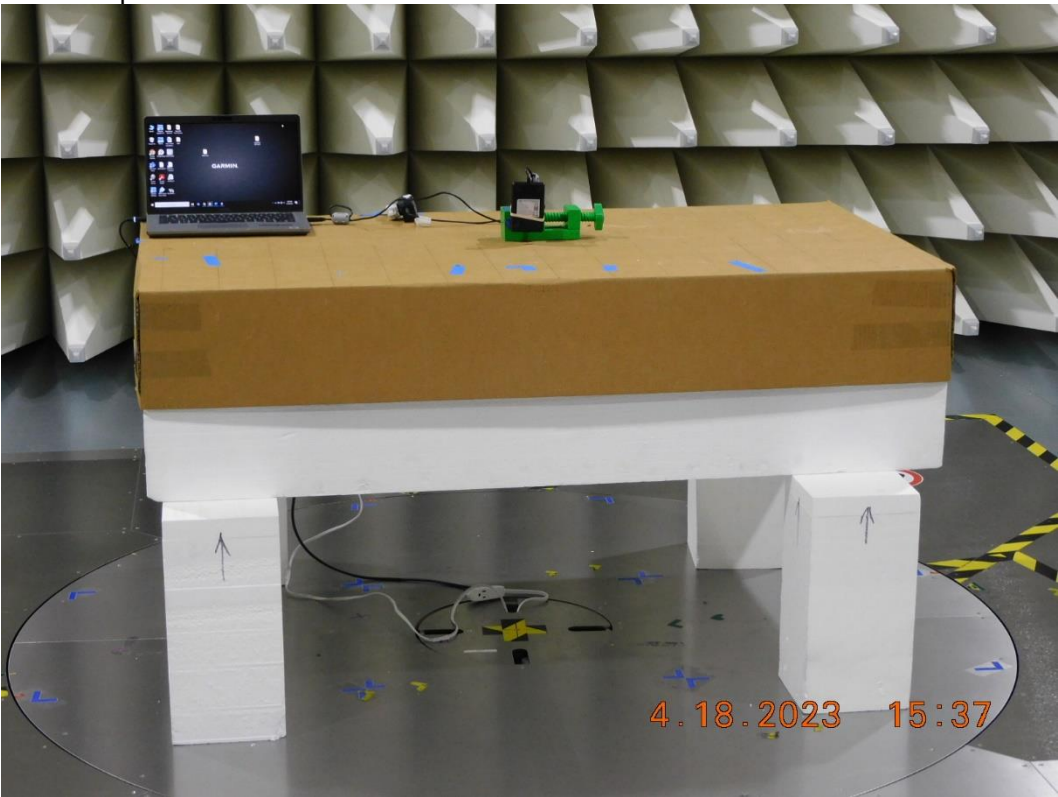
Figure RE014.4: EUT test setup, front view (Antenna X Orientation)
