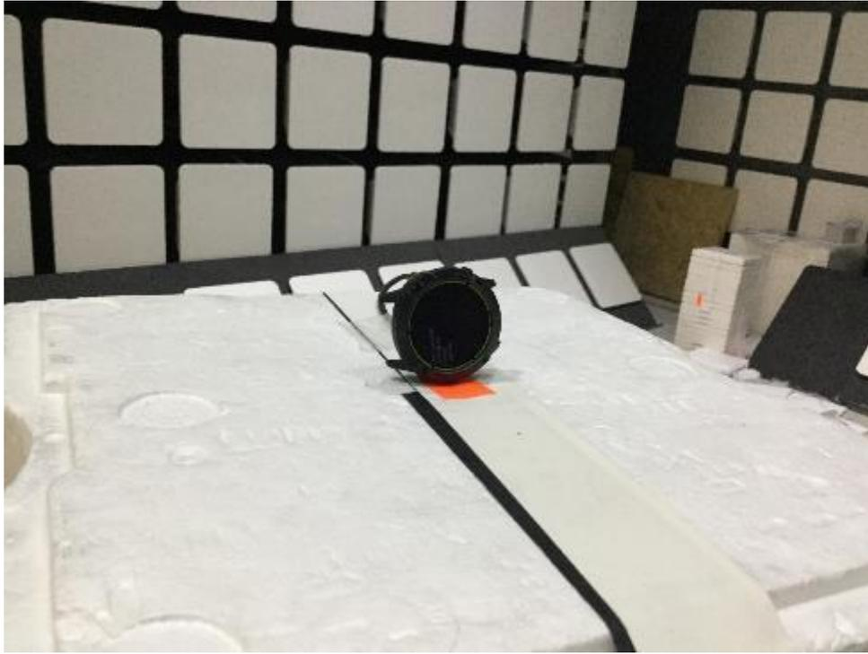
Radiated Emissions Test Setup, 1 - 25 GHz
