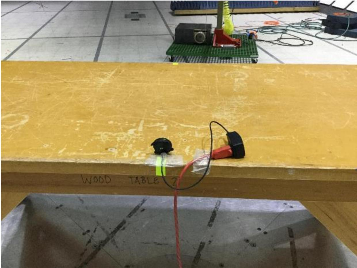
Radiated Emissions Test Setup, 30 MHz - 1 GHz
