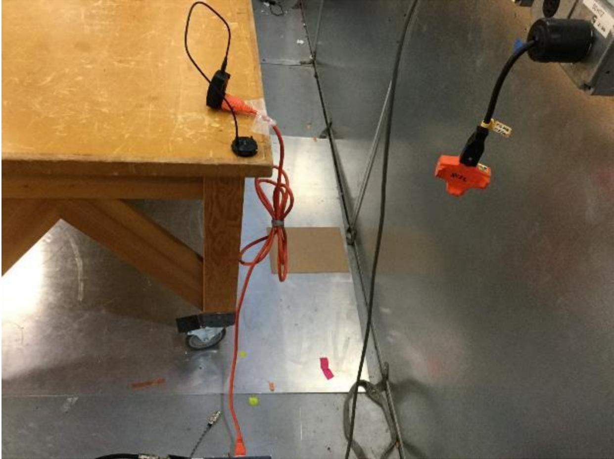
Conducted Emissions Test Setup, 150 kHz – 30 MHz
