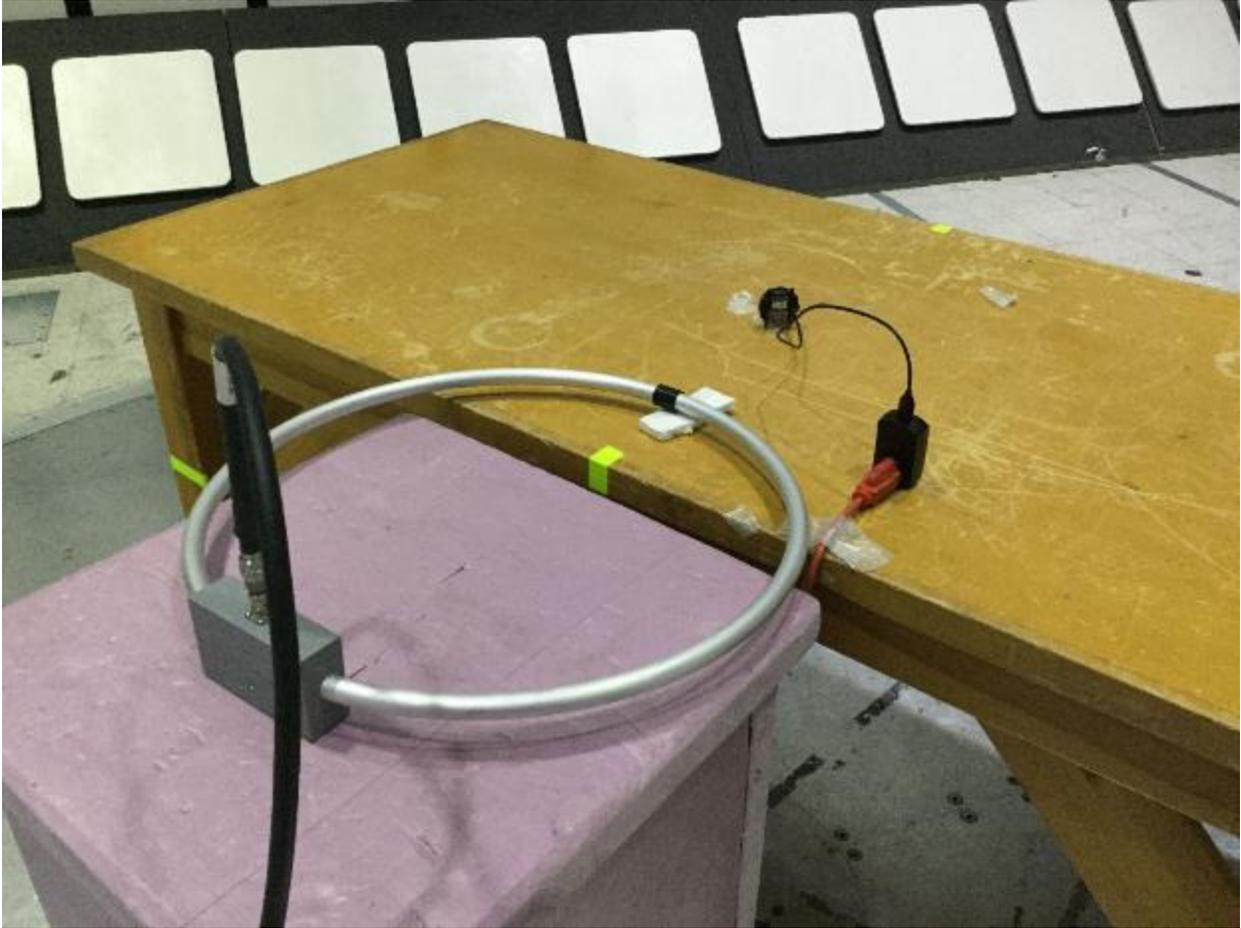
Radiated Emissions Test Setup, 10 - 30 MHz
