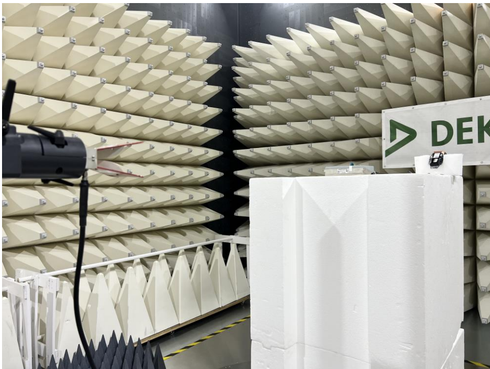
Figure B8. High Range Radiated Emission test setup 2
