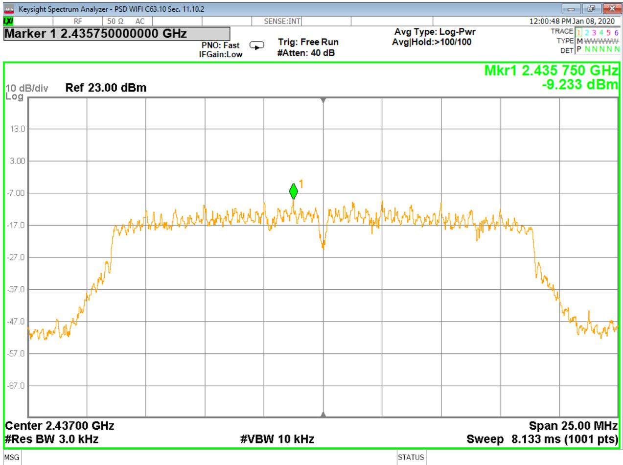
Figure 60 - Power Spectral Density, Mid Channel, 802.11n
