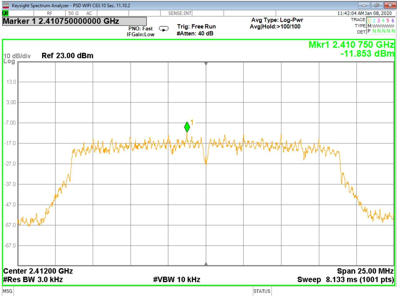
Figure 59 - Power Spectral Density, Low Channel, 802.11n
