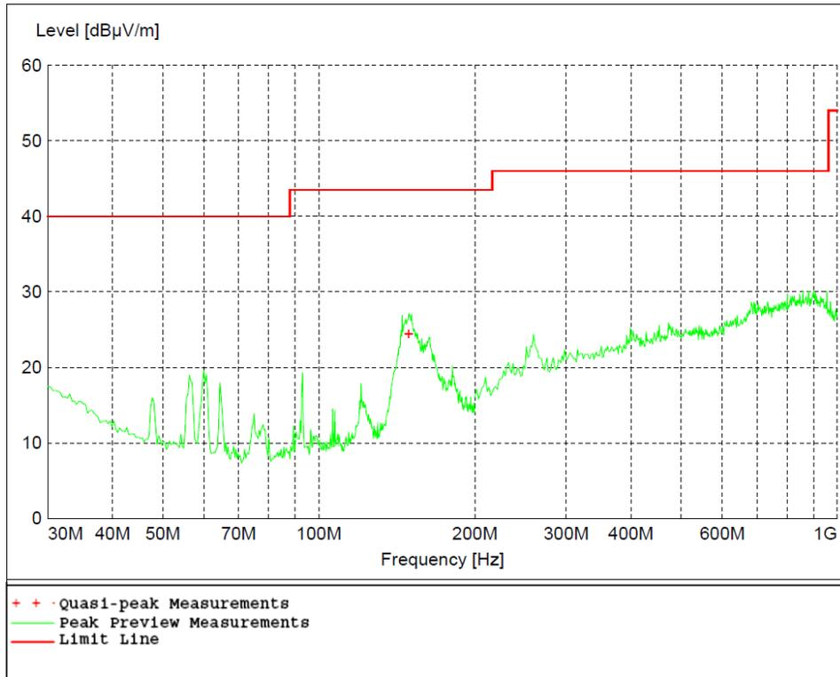
Figure 2 – Radiated Emissions Peak Plot, 30 MHz- 1 GHz
