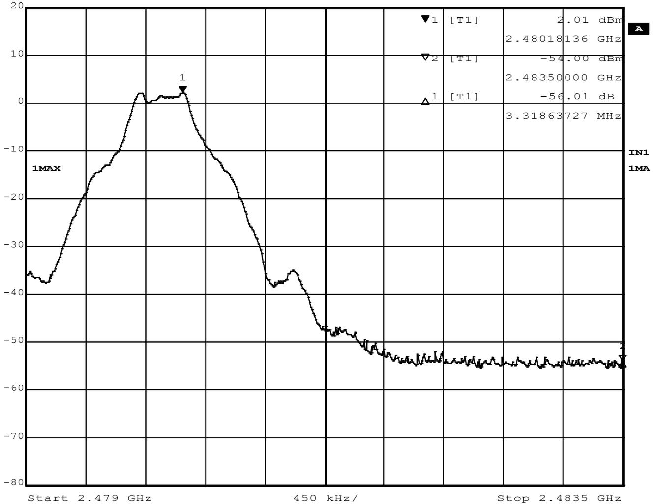
Figure 30 –Band Edge Measurement, High Channel, Unrestricted, GFSK
