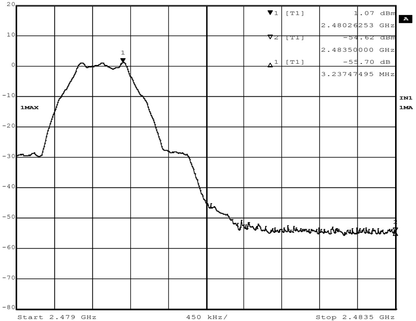
Figure 32 – Band Edge Measurement, High Channel, Unrestricted, GMSK
