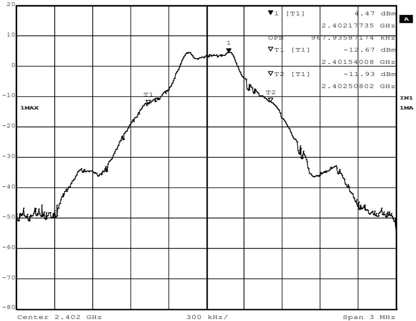
Figure 8 – Occupied Bandwidth, Low Channel, GFSK
