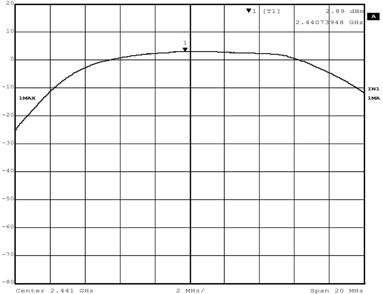
**Figure 2 – Output Power, Mid Channel, GFSK**
