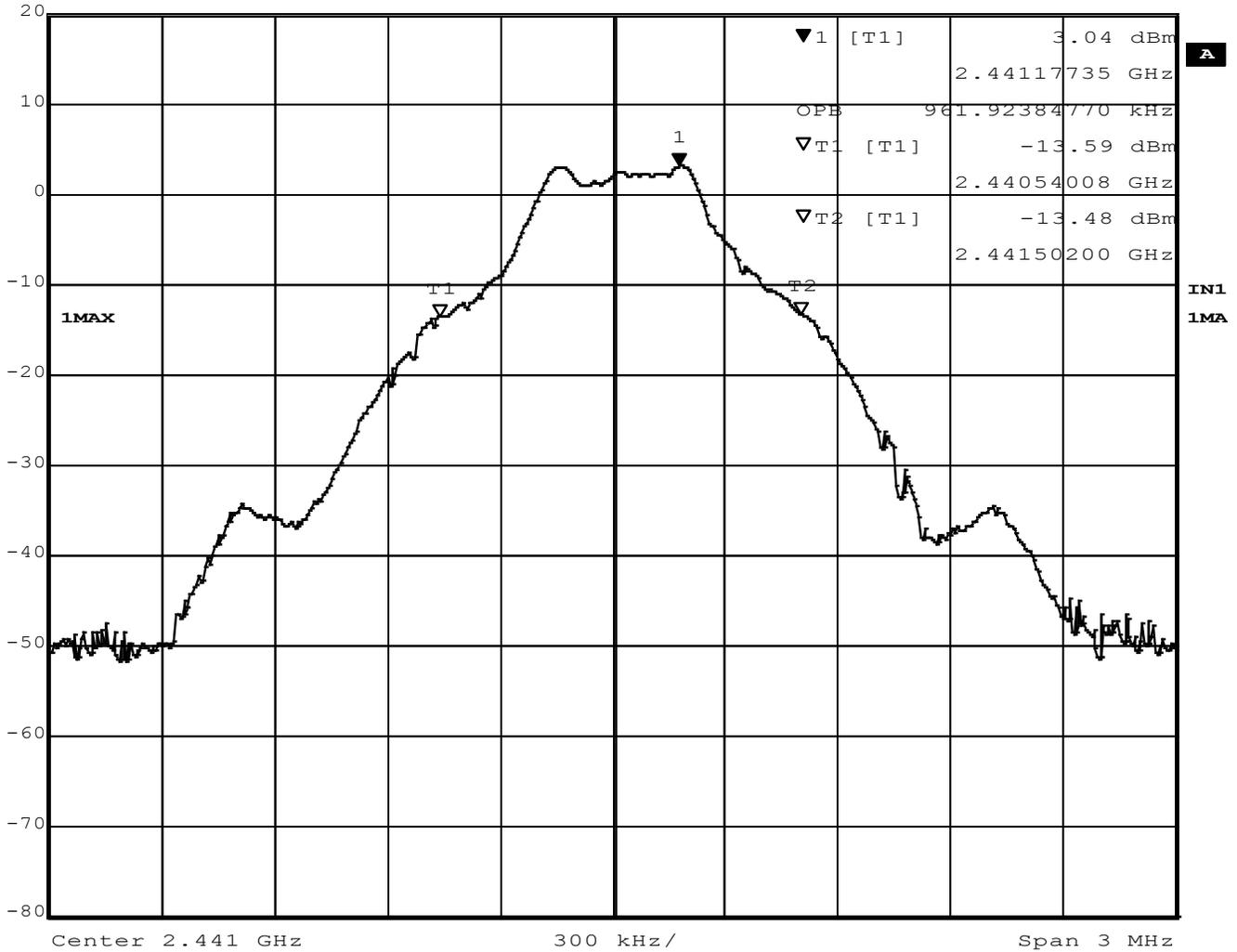
Figure 9 - Occupied Bandwidth, Mid Channel, GFSK
