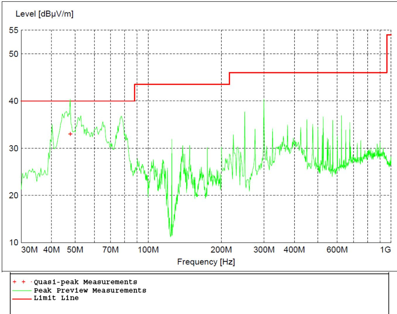
Figure 28 - Radiated Emissions Plot, High Channel, GFSK, 10 Inch Unit
