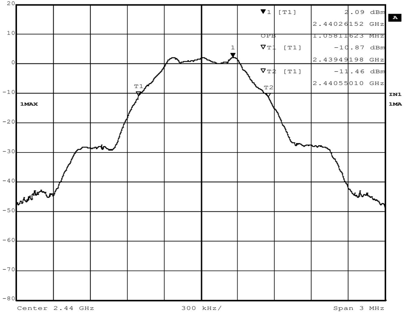
Figure 12 - Occupied Bandwidth, Mid Channel, GMSK
