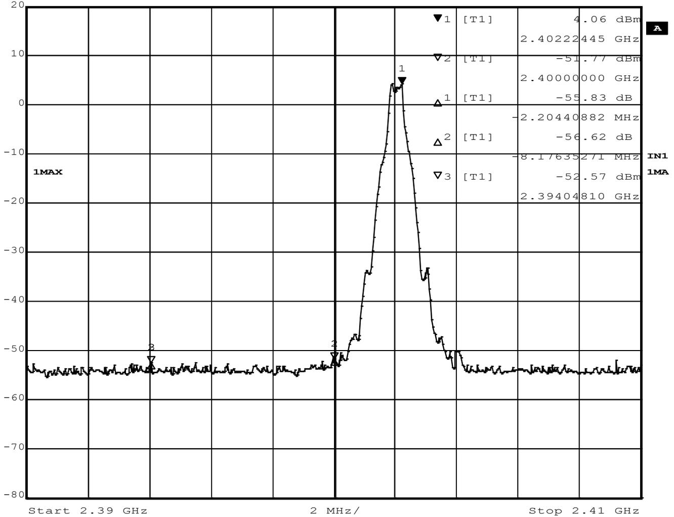
Figure 29 - Band Edge, Low Channel, Unrestricted, GFSK
