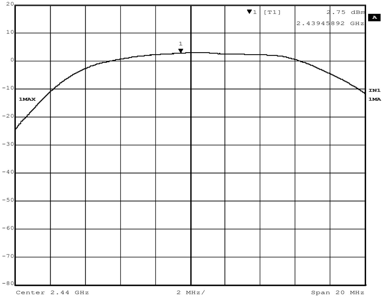
**Figure 5 - Output Power, Mid Channel, GMSK**
