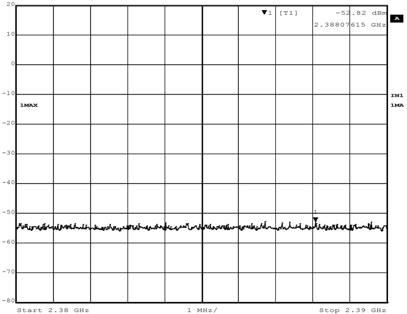
Figure 33 - Band Edge, Low Channel, Restricted, GFSK
