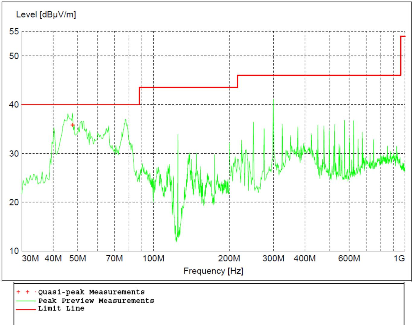
Figure 26 - Radiated Emissions Plot, Low Channel, GFSK, 10 Inch Unit
