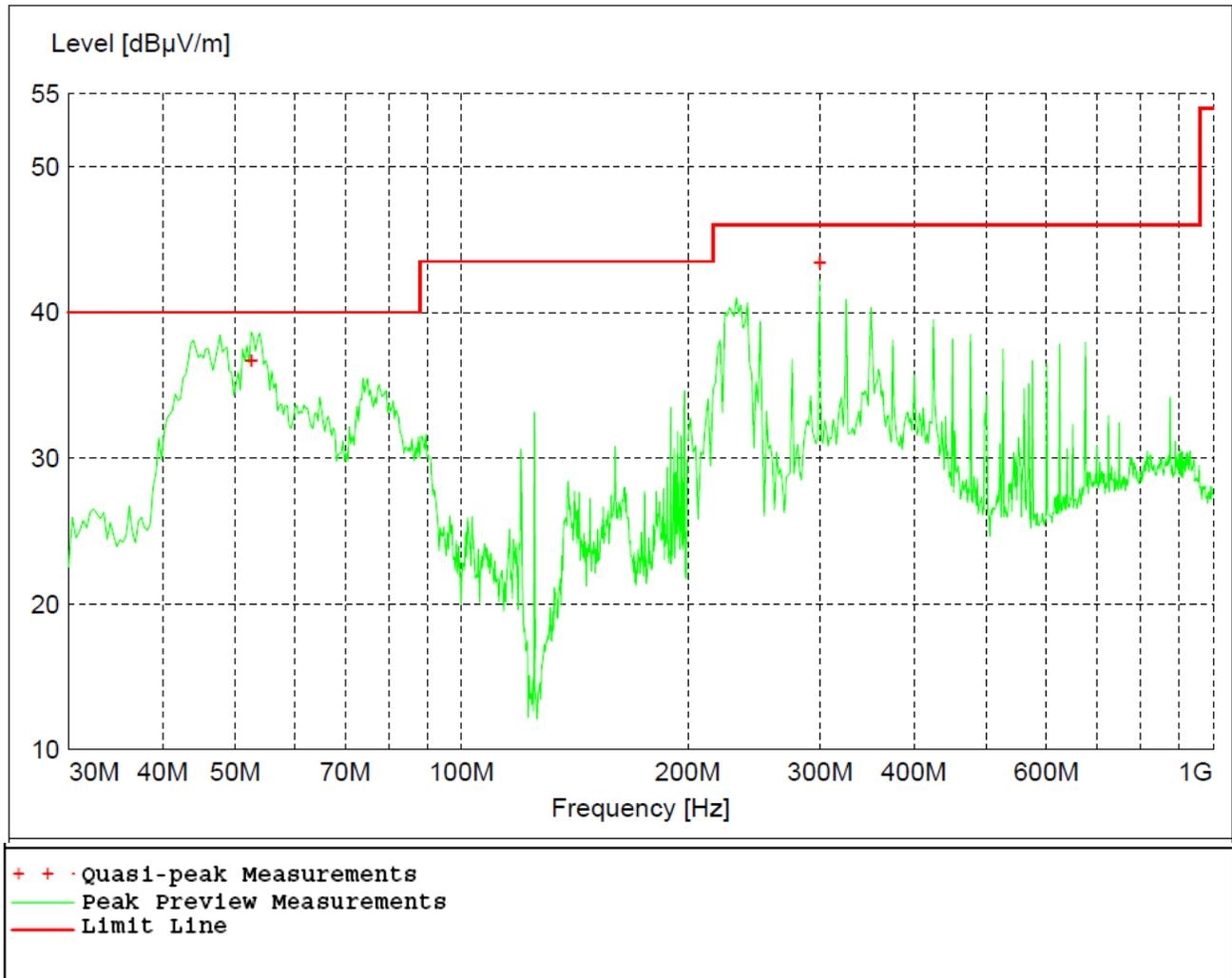
Figure 22 - Radiated Emissions Plot, High Channel, GFSK, 12 Inch Unit
