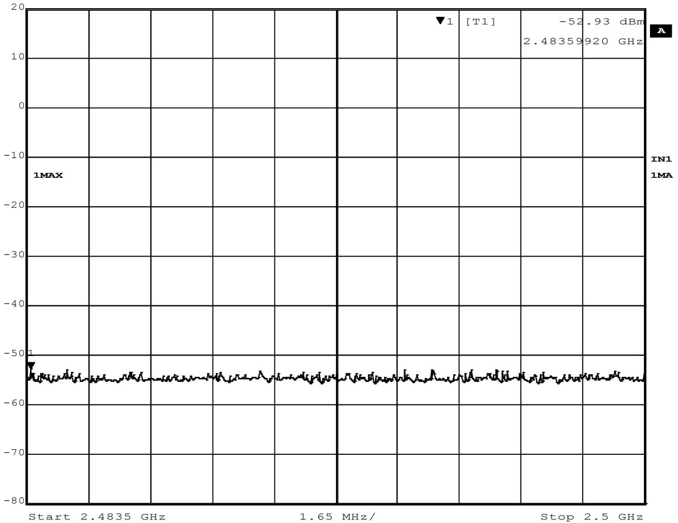
**Figure 34 –Band Edge Measurement, High Channel, Restricted, GFSK**
