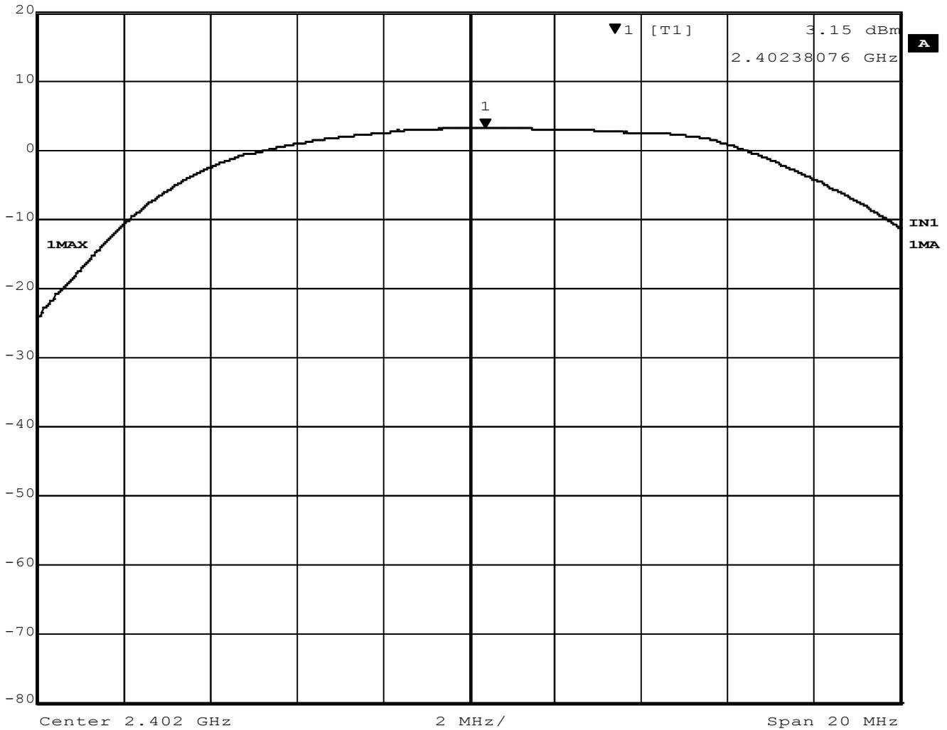
**Figure 4 - Output Power, Low Channel, GMSK**
