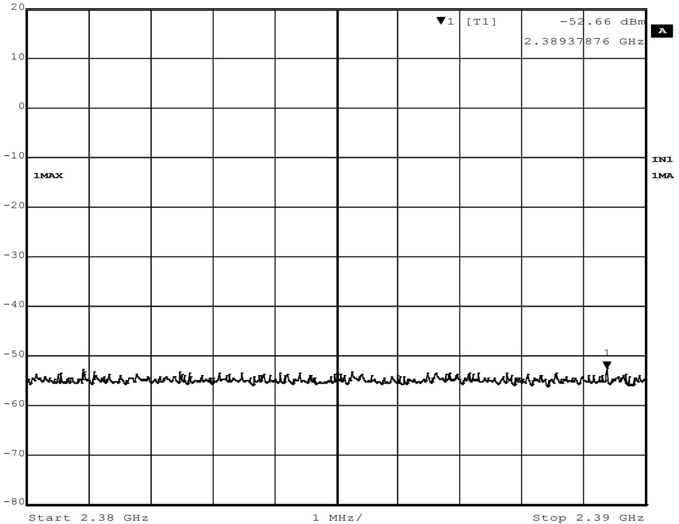
**Figure 35 –Band Edge, Low Channel, Restricted, GMSK**
