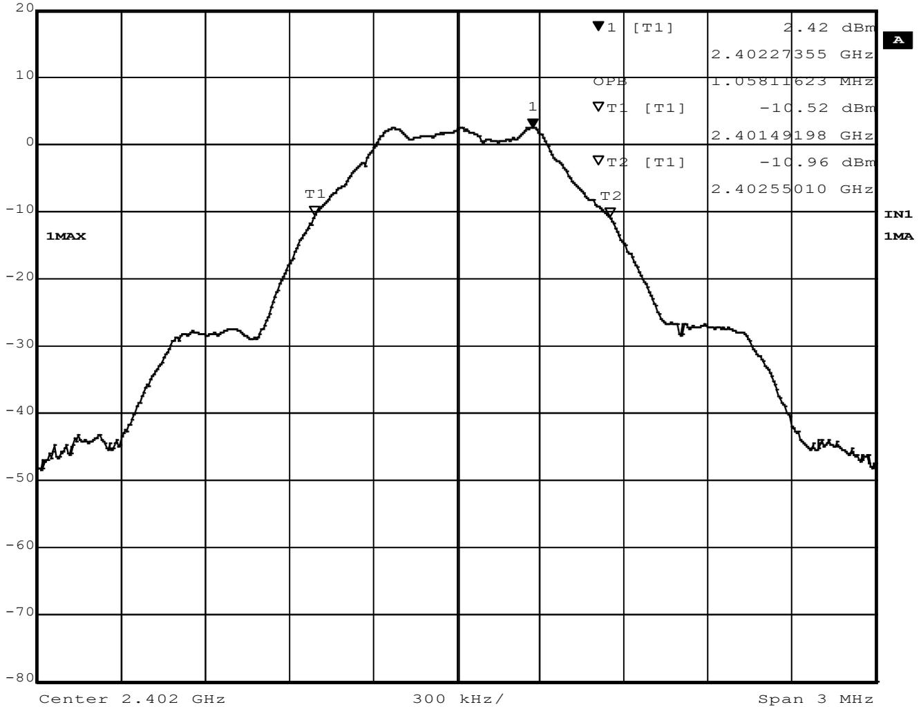
Figure 11 – Occupied Bandwidth, Low Channel, GMSK
