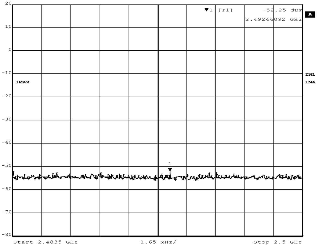
Figure 36 – Band Edge Measurement, High Channel, Restricted, GMSK
