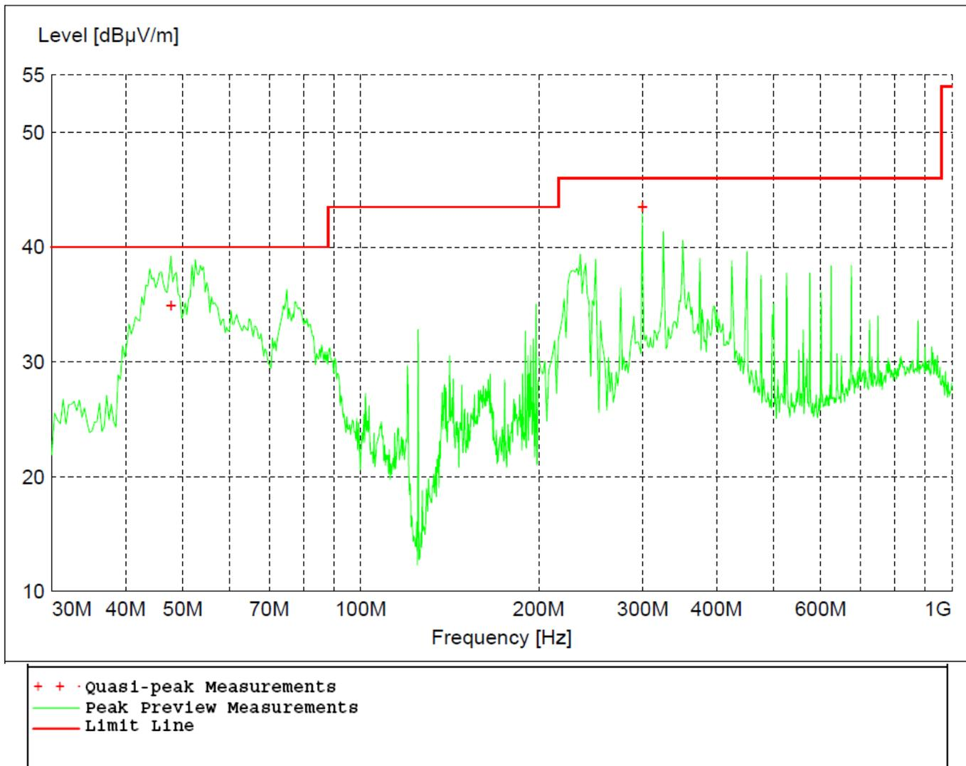
Figure 19 - Radiated Emissions Plot, High Channel, GMSK, 12 Inch Unit
