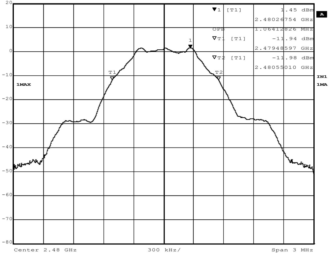
Figure 13 - Occupied Bandwidth, High Channel, GMSK
