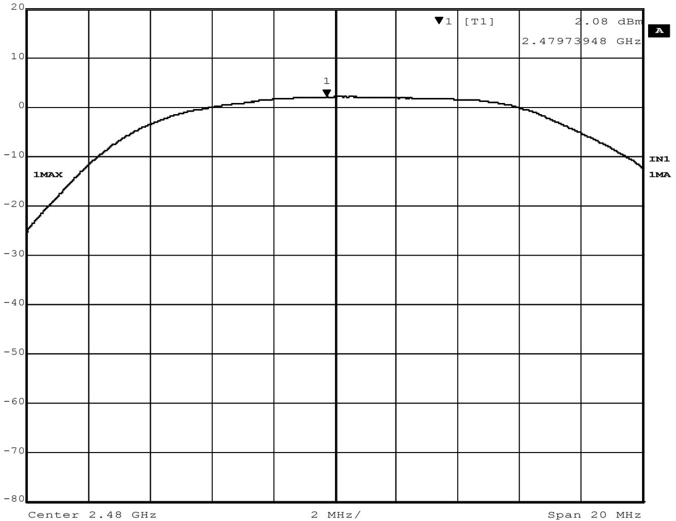
**Figure 6 - Output Power, High Channel, GMSK**
