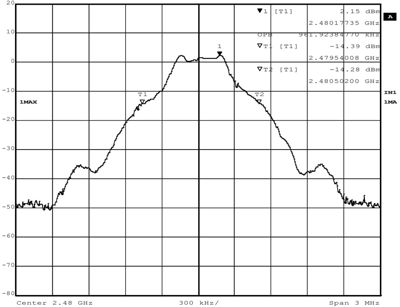
Figure 10 - Occupied Bandwidth, High Channel, GFSK
