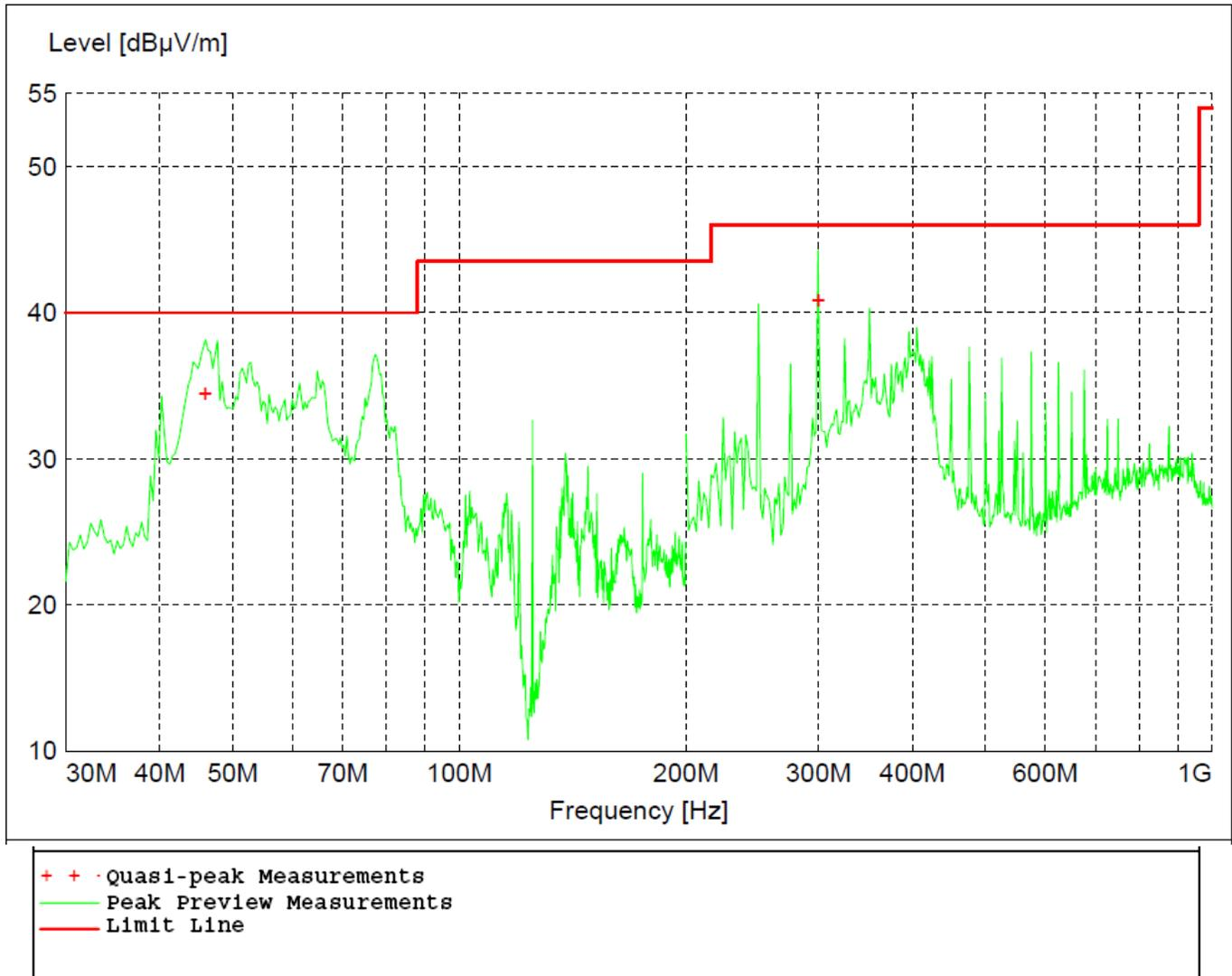
Figure 23 - Radiated Emissions Plot, Low Channel, GMSK, 10 Inch Unit
