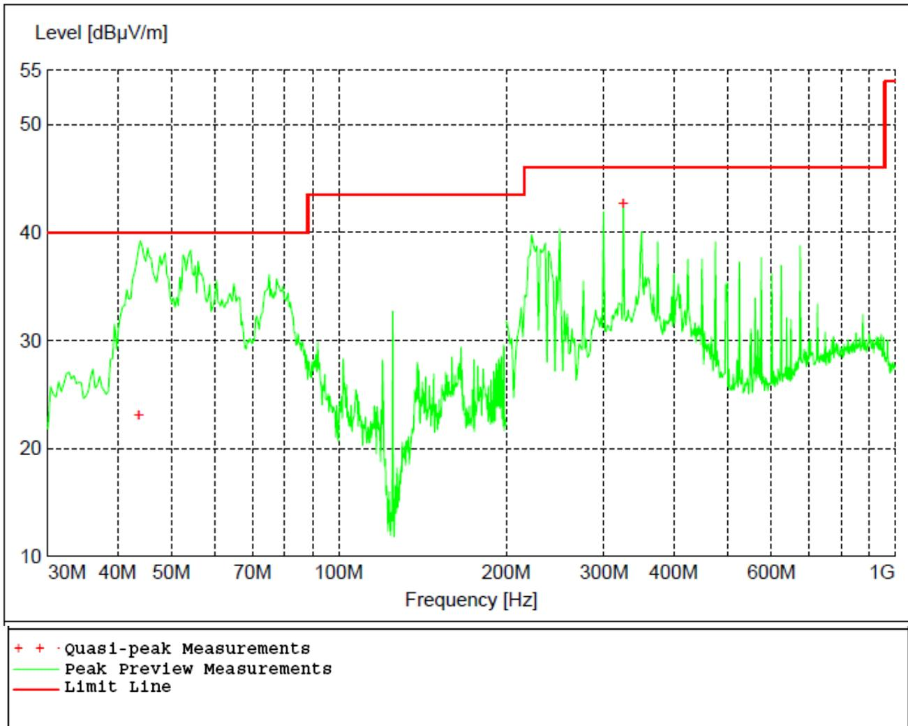
Figure 17 - Radiated Emissions Plot, Low Channel, GMSK, 12 Inch Unit
