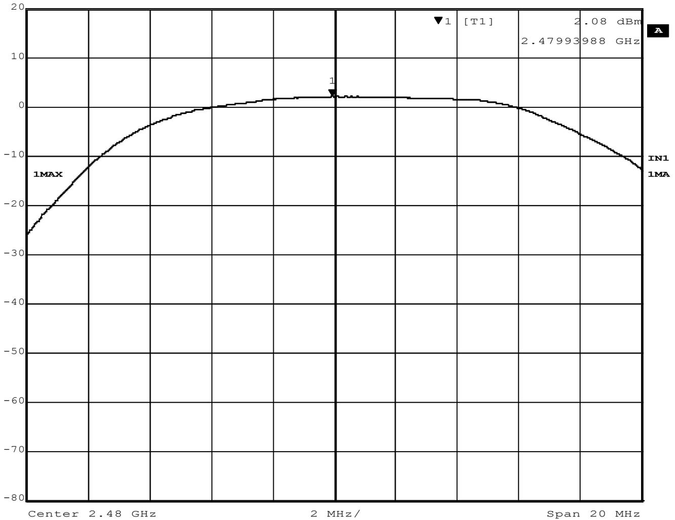
**Figure 3 – Output Power, High Channel, GFSK**
