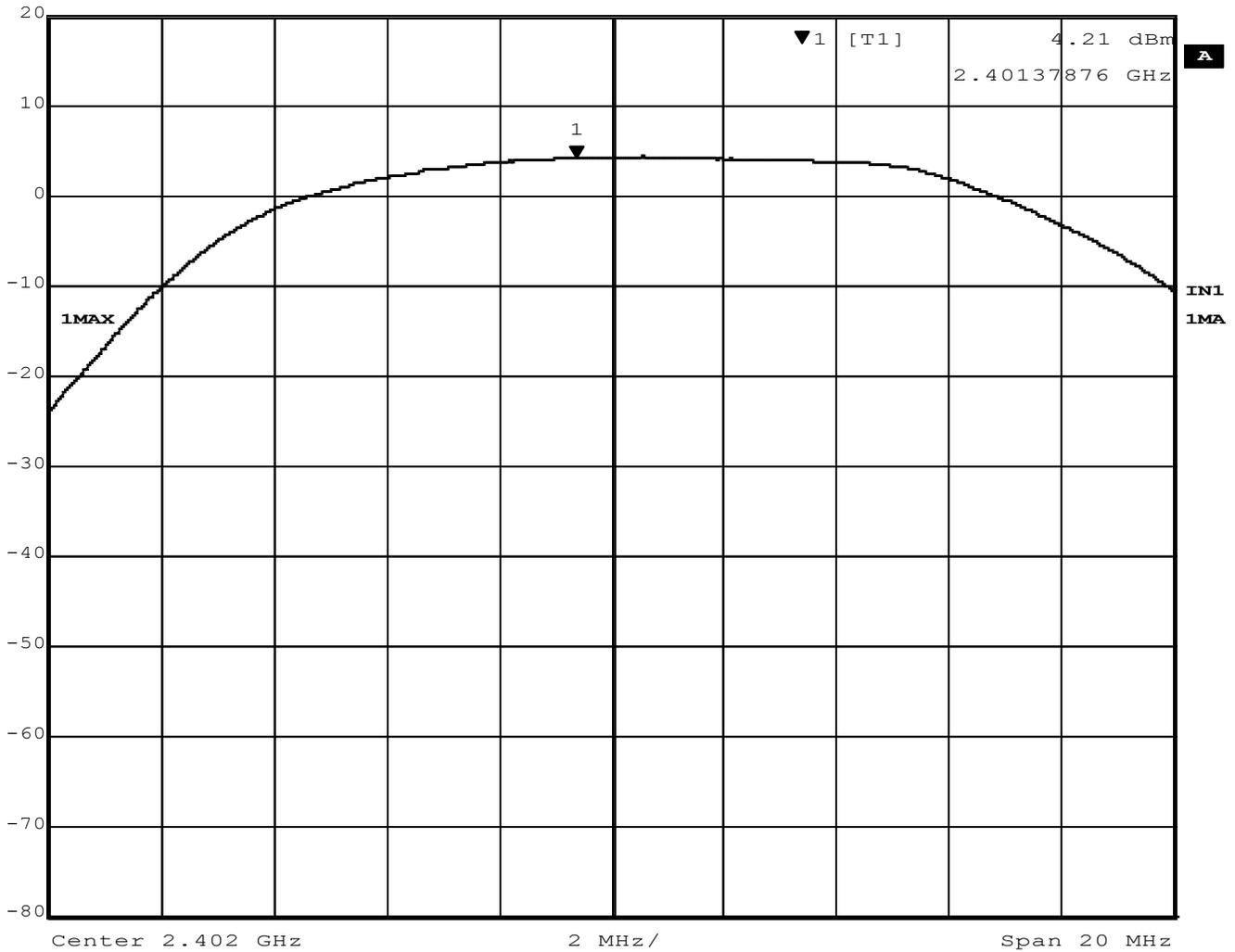
Figure 1 – Output Power, Low Channel, GFSK
