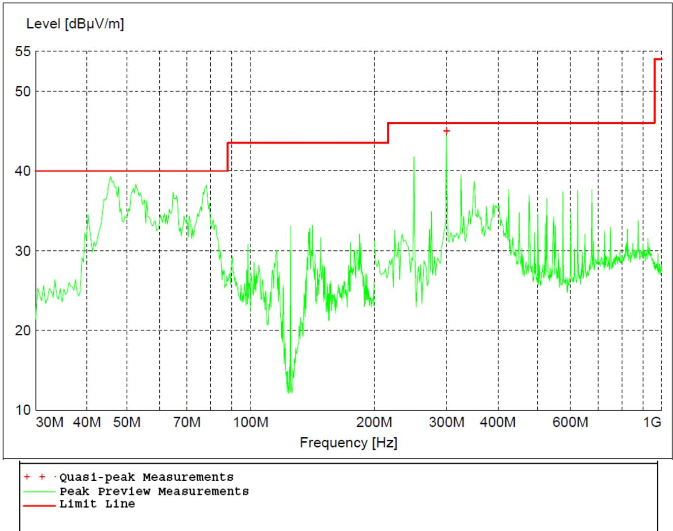
Figure 16 - Radiated Emissions Plot, Receive, 10 Inch Unit
