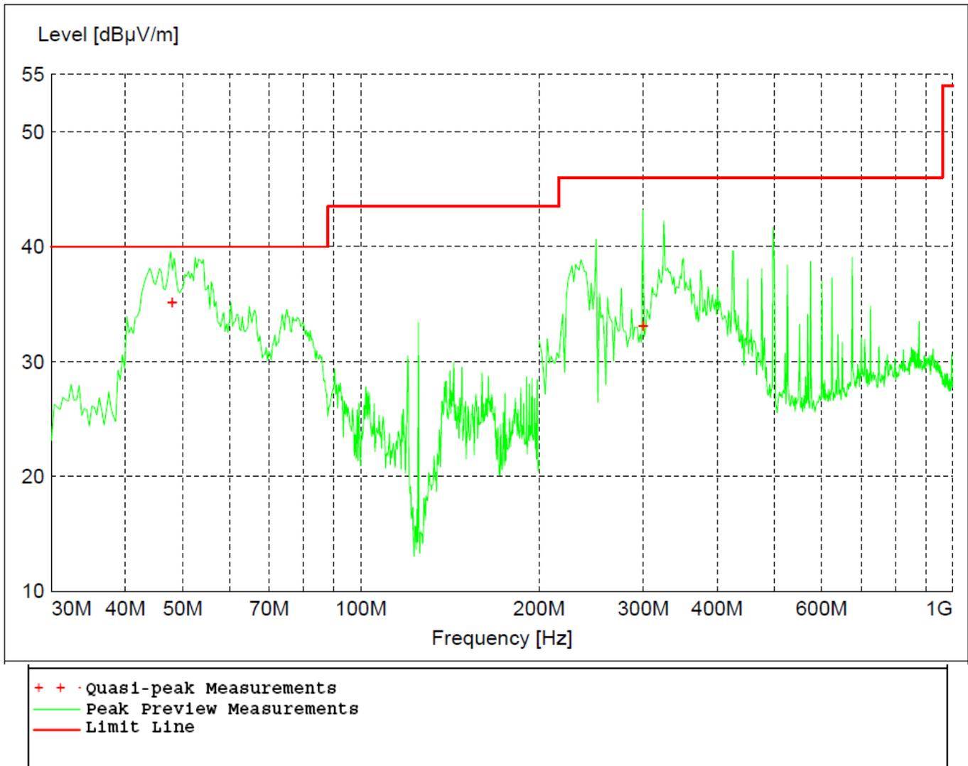
**Figure 15 - Radiated Emissions Plot, Receive, 12 Inch Unit**
