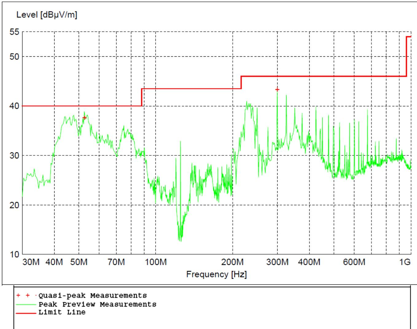
Figure 20 - Radiated Emissions Plot, Low Channel, GFSK, 12 Inch Unit
