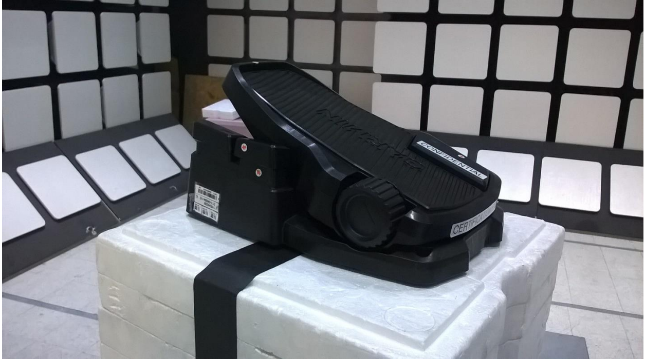
Radiated emissions test setup, 1 – 25 GHz
