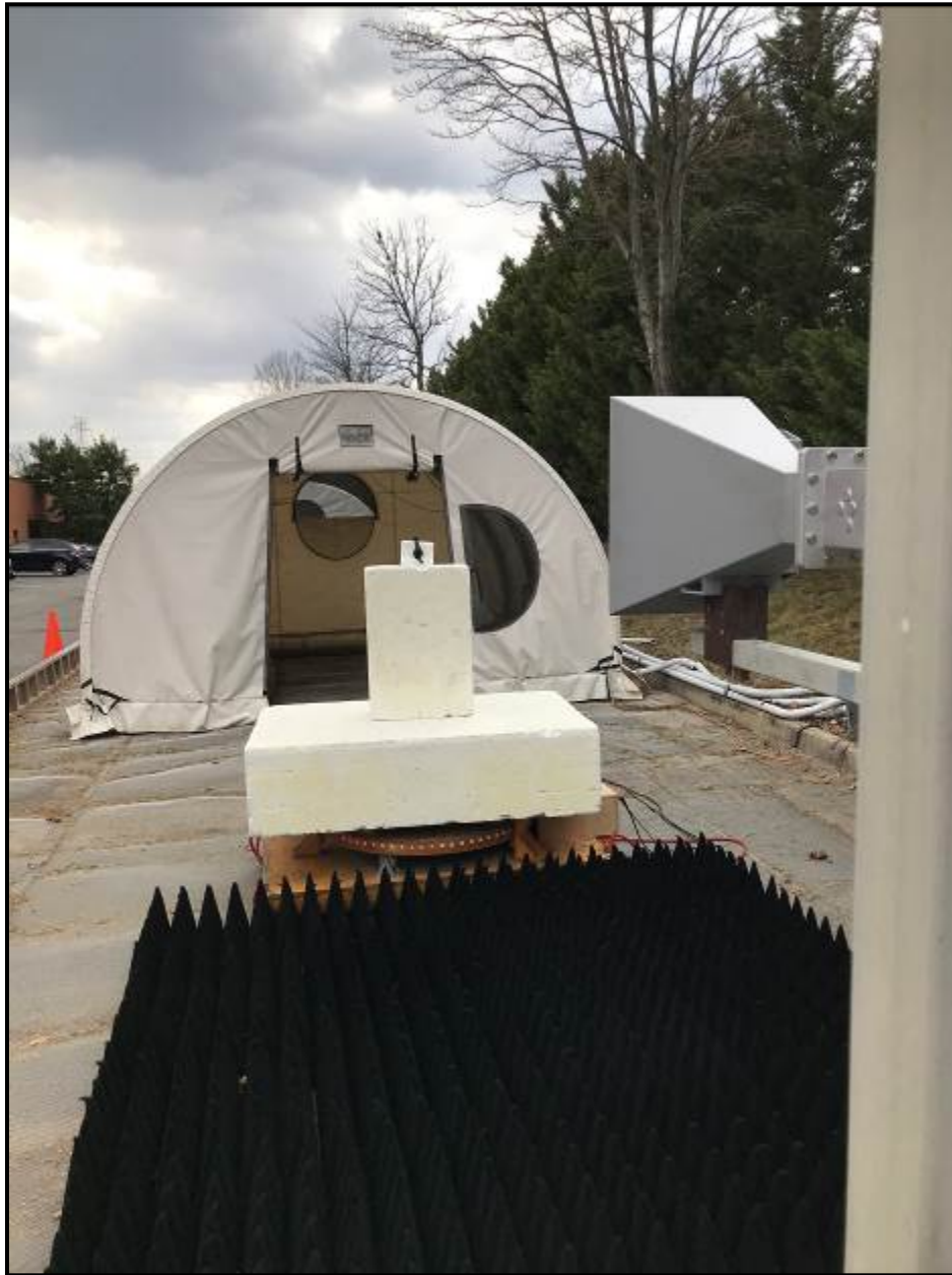
Photograph 1: Radiated Emissions Testing – Front View (Above 1 GHz)
