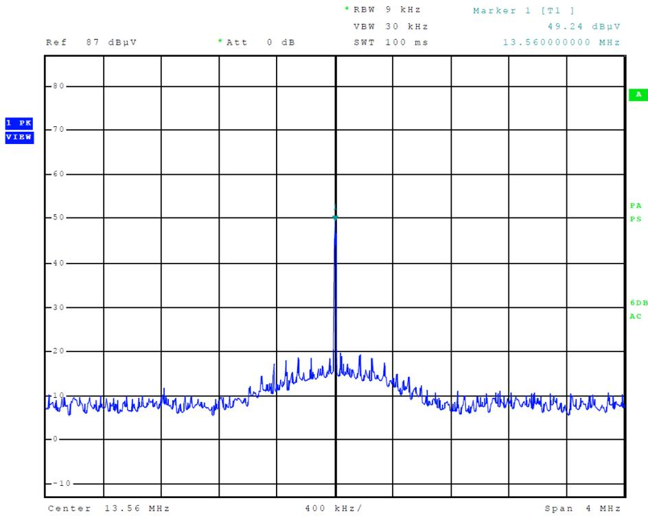
**Figure 7 Plot of NFC Operation Across Frequency Spectrum**
