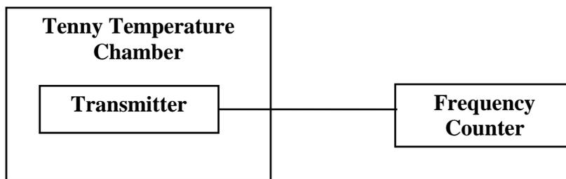
The measurement procedure outlined below shall be followed during measurement of frequency variation over temperature.
