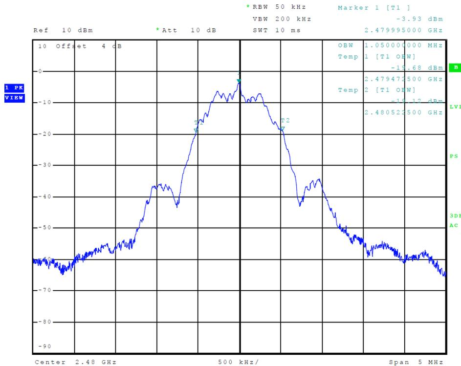
Figure 12 Plot of Transmitter Emissions (99% Occupied Bandwidth, BLE)
