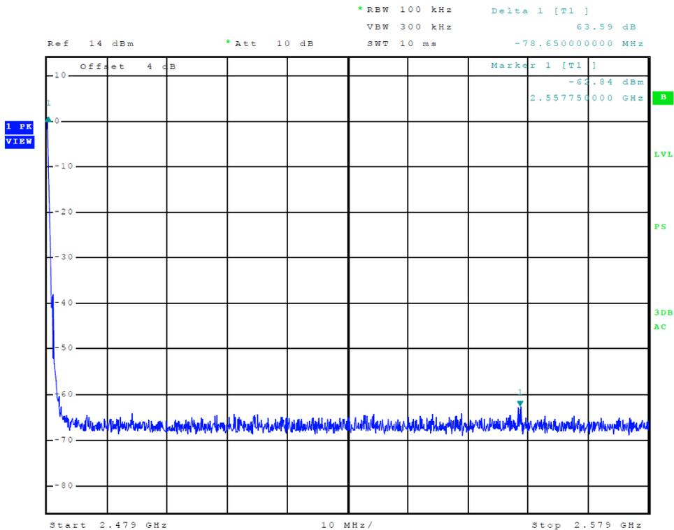
**Figure 6 Plot of Transmitter Emissions (High Band Edge, GFSK)**
