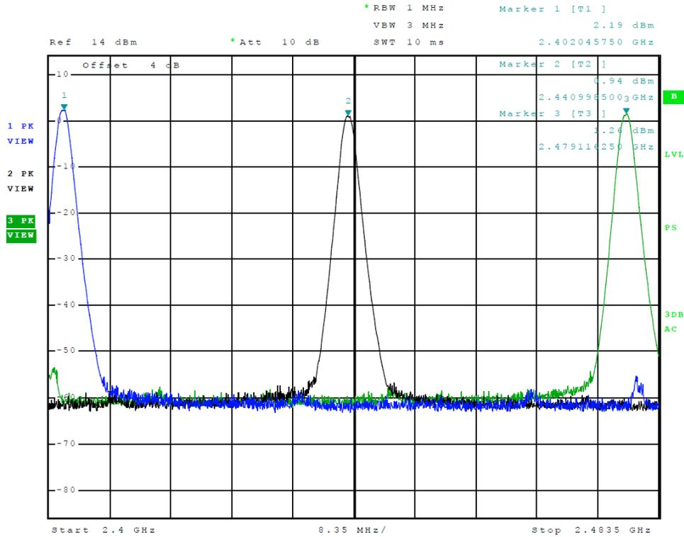
**Figure 3 Plot of Transmitter Emissions (Operation in 2402-2479 MHz. GFSK)**
