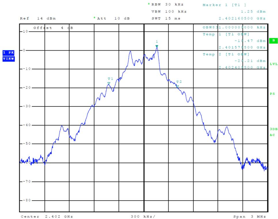
**Figure 4 Plot of Transmitter Emissions (99% Occupied Bandwidth, GFSK)**
