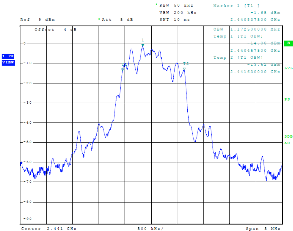
Figure 12 Plot of Transmitter Emissions (99% Occupied Bandwidth, \pi/4 DQPSK)
