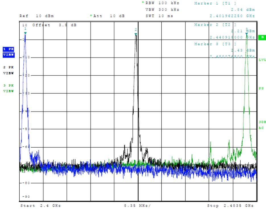
Figure 3 Plot of Transmitter Emissions (In 2402-2480 MHz Band) (Mode 1)
