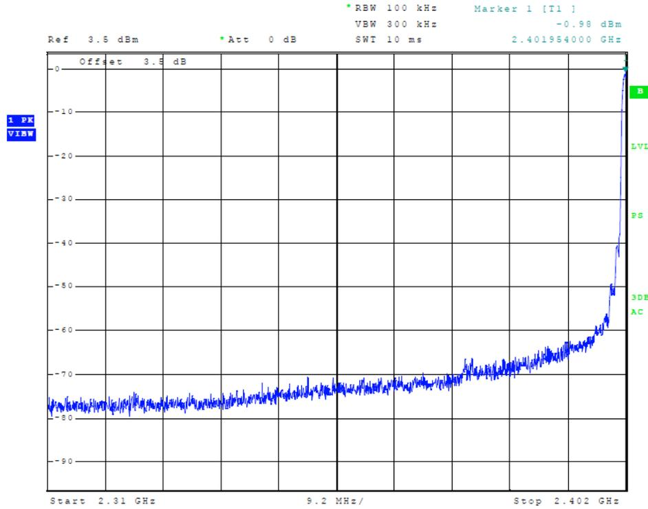
Figure 13 Plot of Transmitter Emissions (Low Band Edge) (Mode 2, 3MB)
