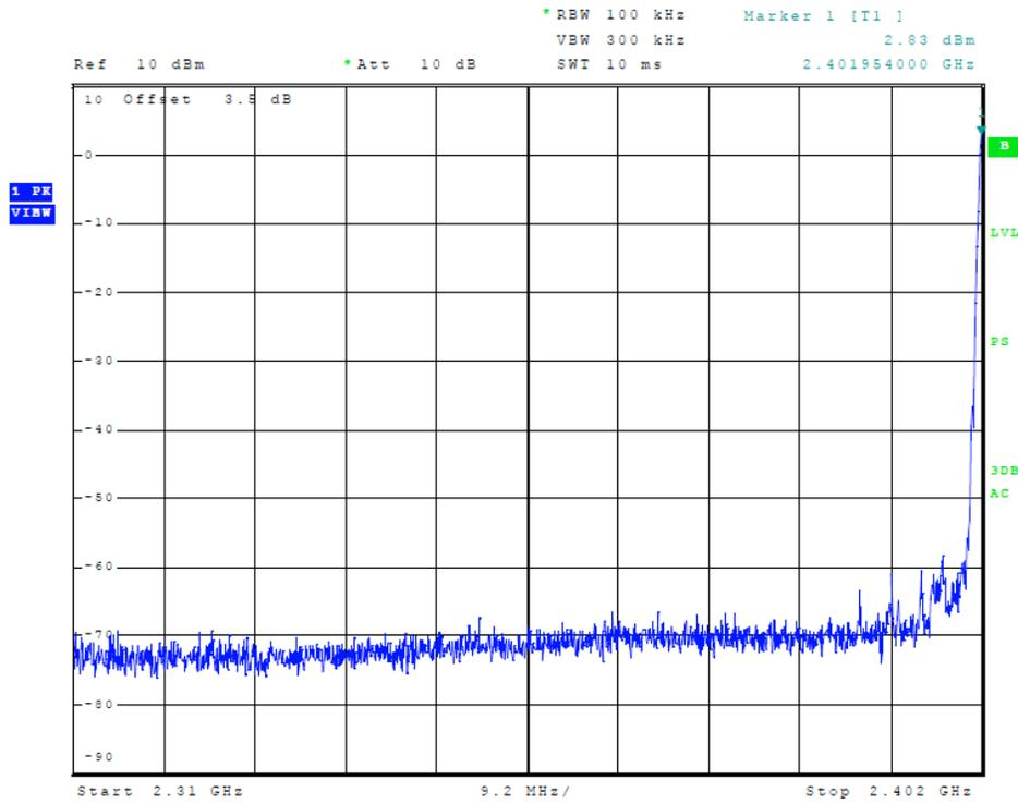
Figure 5 Plot of Transmitter Emissions (Low Band Edge) (Mode 1)
