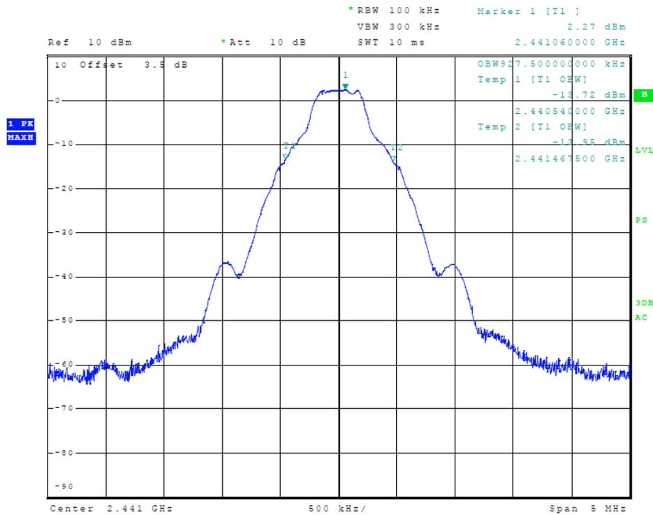
Figure 4 Plot of Transmitter Emissions (99% Occupied Bandwidth) (Mode 1)
