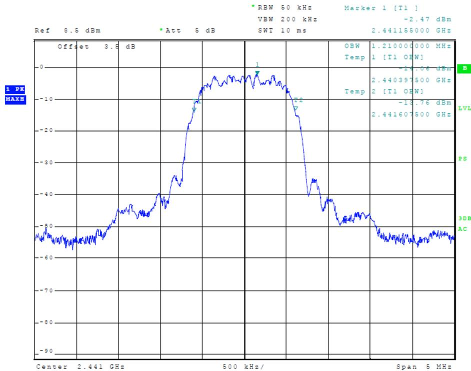
**Figure 8 Plot of Transmitter Emissions (99% Occupied Bandwidth) (Mode 2, 2MB)**
