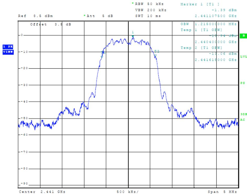
Figure 12 Plot of Transmitter Emissions (99% Occupied Bandwidth) (Mode 2, 3MB)
