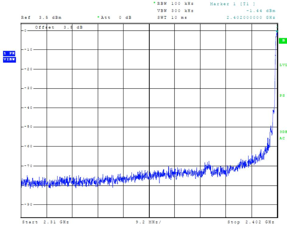
**Figure 9 Plot of Transmitter Emissions (Low Band Edge) (Mode 2, 2MB)**
