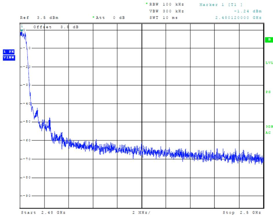
Figure 14 Plot of Low Band Edge (High Band Edge) (Mode 2, 3MB)
