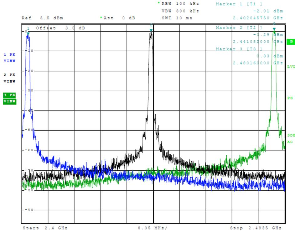
Figure 11 Plot of Transmitter Emissions (In 2402-2480 MHz Band) (Mode 2, 3MB)
