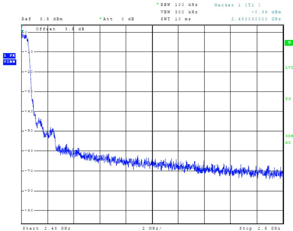
**Figure 10 Plot of Low Band Edge (High Band Edge) (Mode 2, 2MB)**
