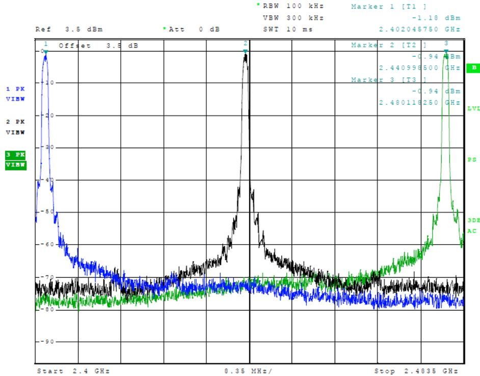
**Figure 7 Plot of Transmitter Emissions (In 2402-2480 MHz Band) (Mode 2, 2MB)**
