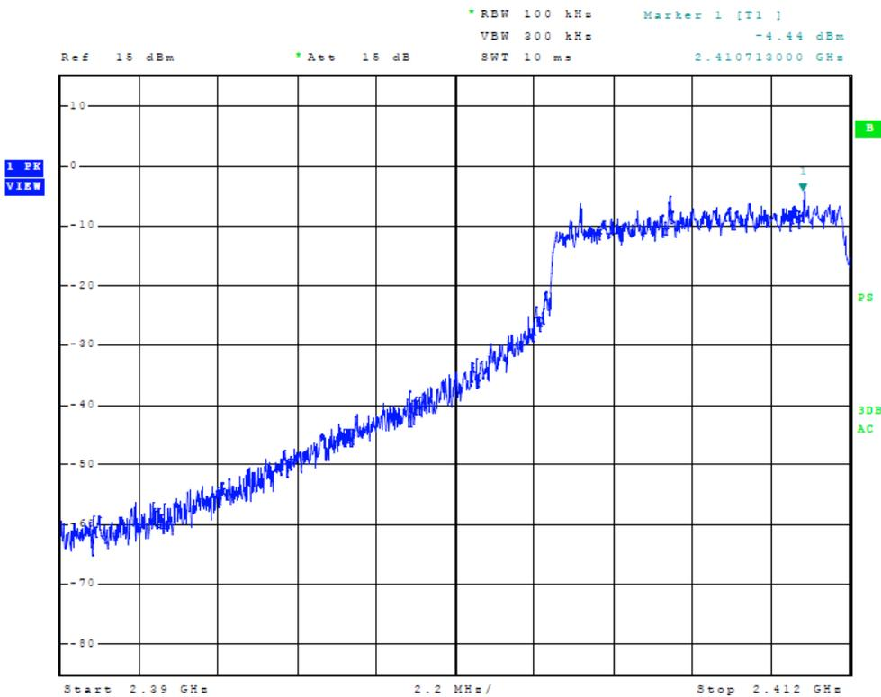
**Figure 6 Plot of Low Band Edge (802.11 G-Mode)**
