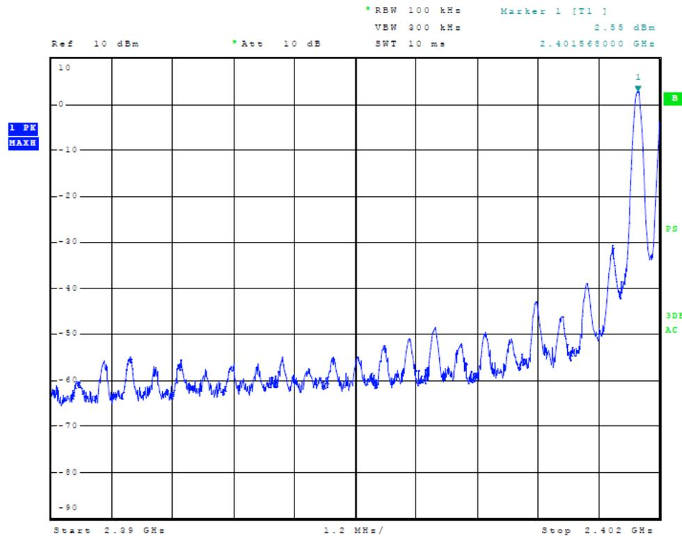
**Figure 8 Plot of Low Band Edge (DTS-Mode)**
