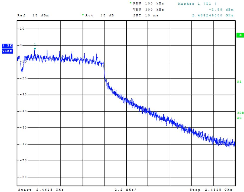
**Figure 7 Plot of High Band Edge (802.11 G-Mode)**
