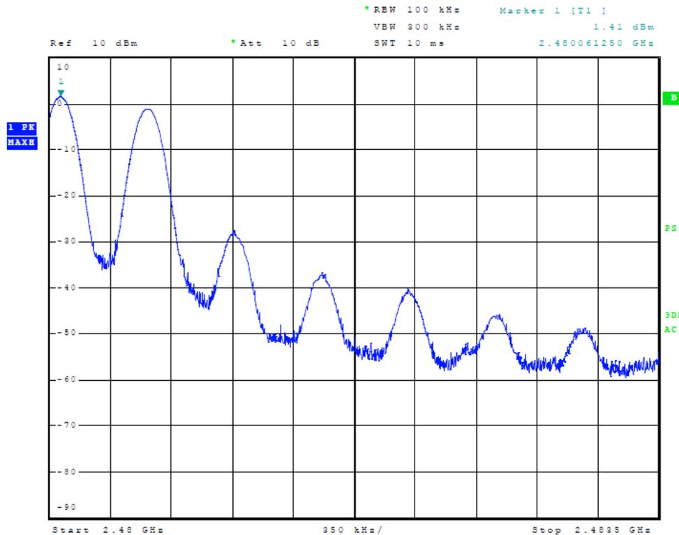
**Figure 9 Plot of High Band Edge (DTS-Mode)**
