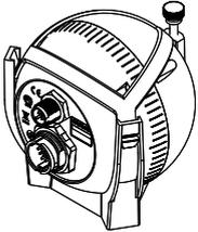
The CCU acts as the “brain” of the GHP 10. The CCU contains the sensory equipment used to determine heading and engine speed. The CCU connects to the Electronic Control Unit (ECU), to the GHC 10, and to the tachometer of your boat with a single cable. The CCU also connects to a NMEA 2000® network to communicate with the GHC 10, and to an optional NMEA 2000-compatible GPS device.
