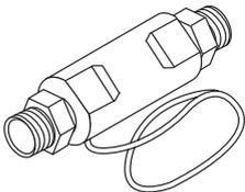
The Shadow Drive is a sensor you install in the hydraulic steering lines of your boat. While the GHP 10 is engaged, the Shadow Drive temporarily disengages the autopilot when you manually take control of the helm. When you manually steer the boat in a straight line again, the Shadow Drive allows the autopilot to resume control.
