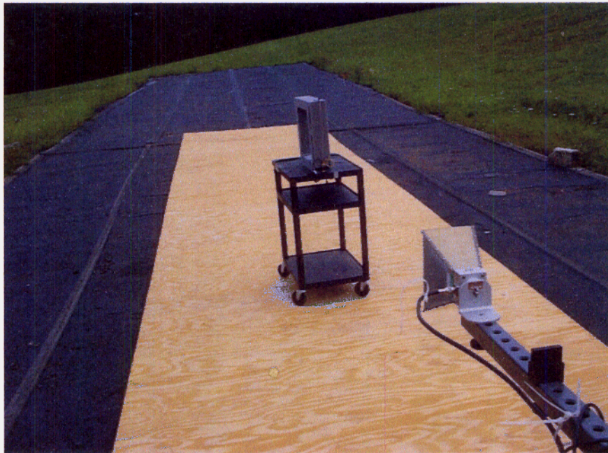
b.) Radiated Emissions test setup
