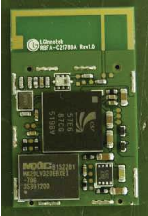
BT Transmitter 3 (without shield case)
