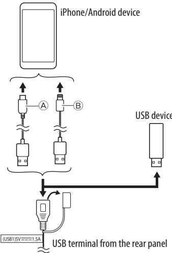
Ⓐ For connecting your Android device, use the USB cable (commercially available)
