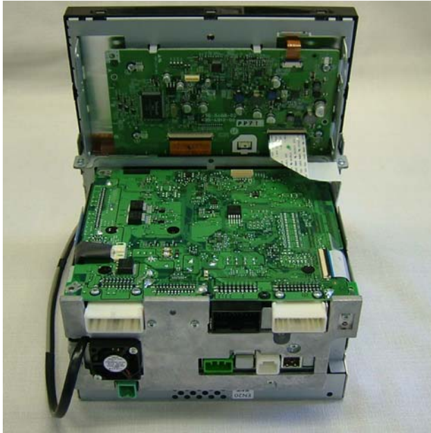
TOP COVER Disassembly
