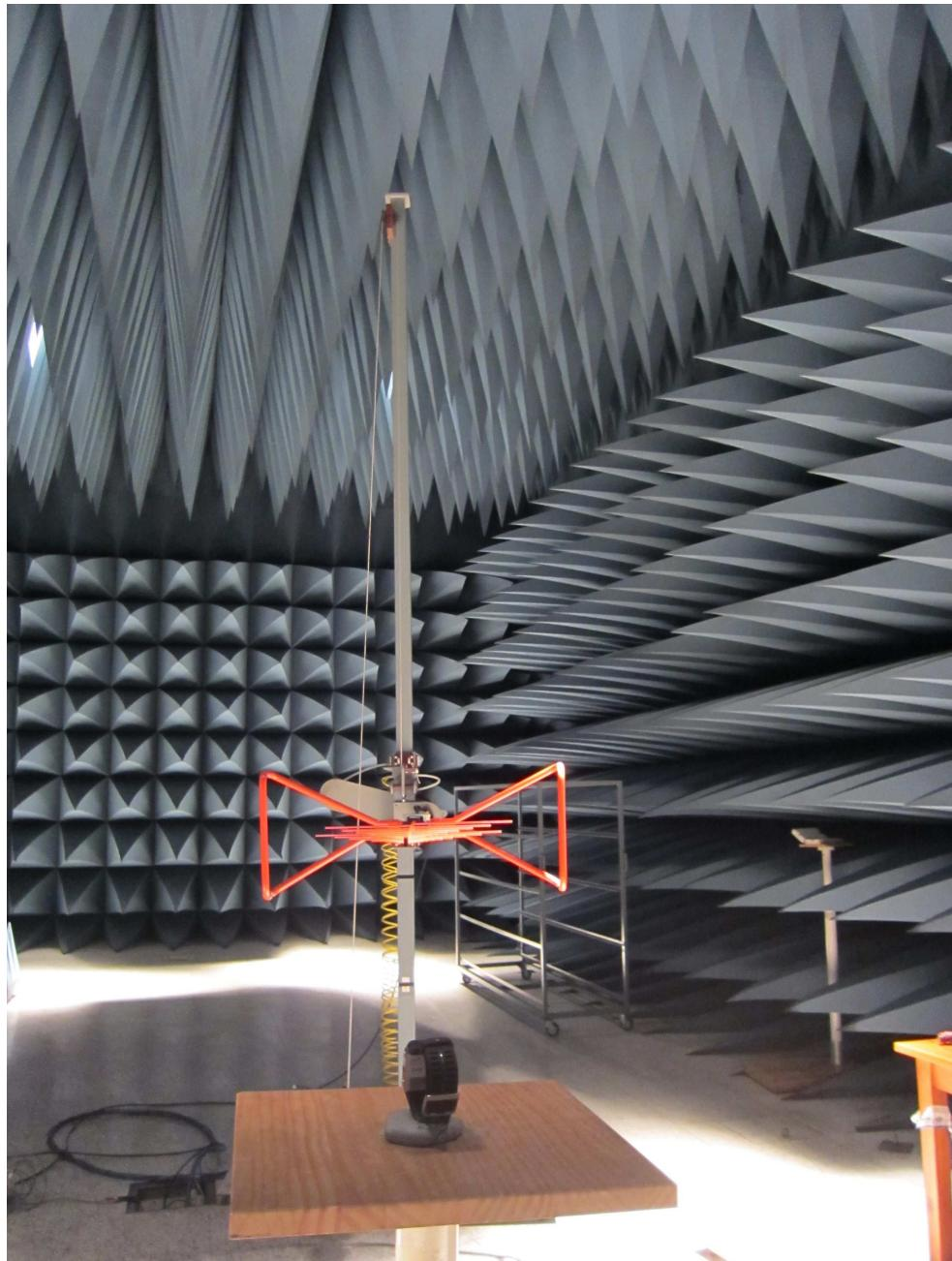
**TEST SET-UP FOR RADIATED MEASUREMENTES ABOVE 1GHz**
