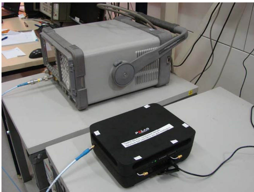
Picture 1: Conducted measurement test setup
