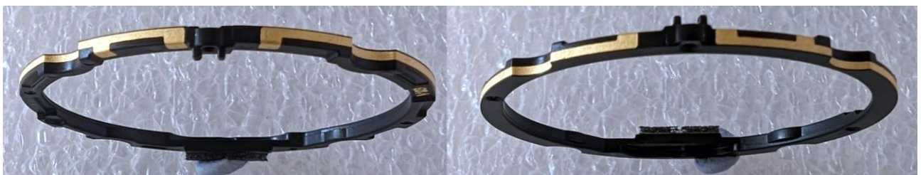
Figure 5. Close-ups of antenna frame.
