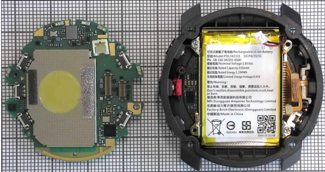
Figure 6. The main PWB removed, device battery visible.
