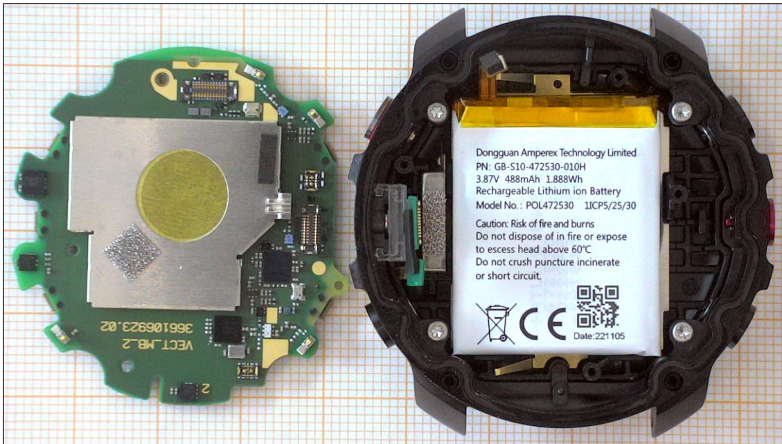
Figure 4. The main PWB removed, device battery visible.
