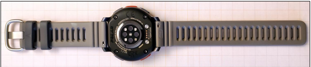
Figure 2. Device from behind, OHR and USB charging cable contacts are visible.
