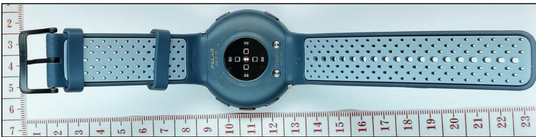
Figure 2. Device from behind, OHR and USB charging cable contacts are visible.
